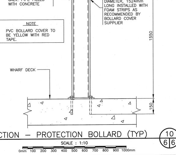
SECTION - PROTECTION BOLLARD (TYP) 10/6/6
