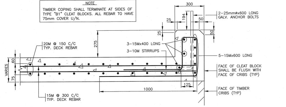
SECTION - TYPE "B1" MOORING CLEAT BLOCK & DECK REBAR 1/6/6
