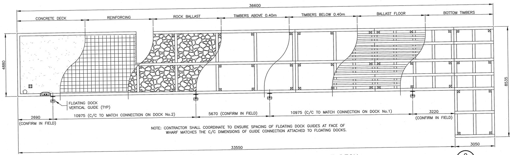
PLAN - MARGINAL WHARF TIMBER CRIB LAYOUT @ BOTTOM TIMBERS TO TOP OF DECK
