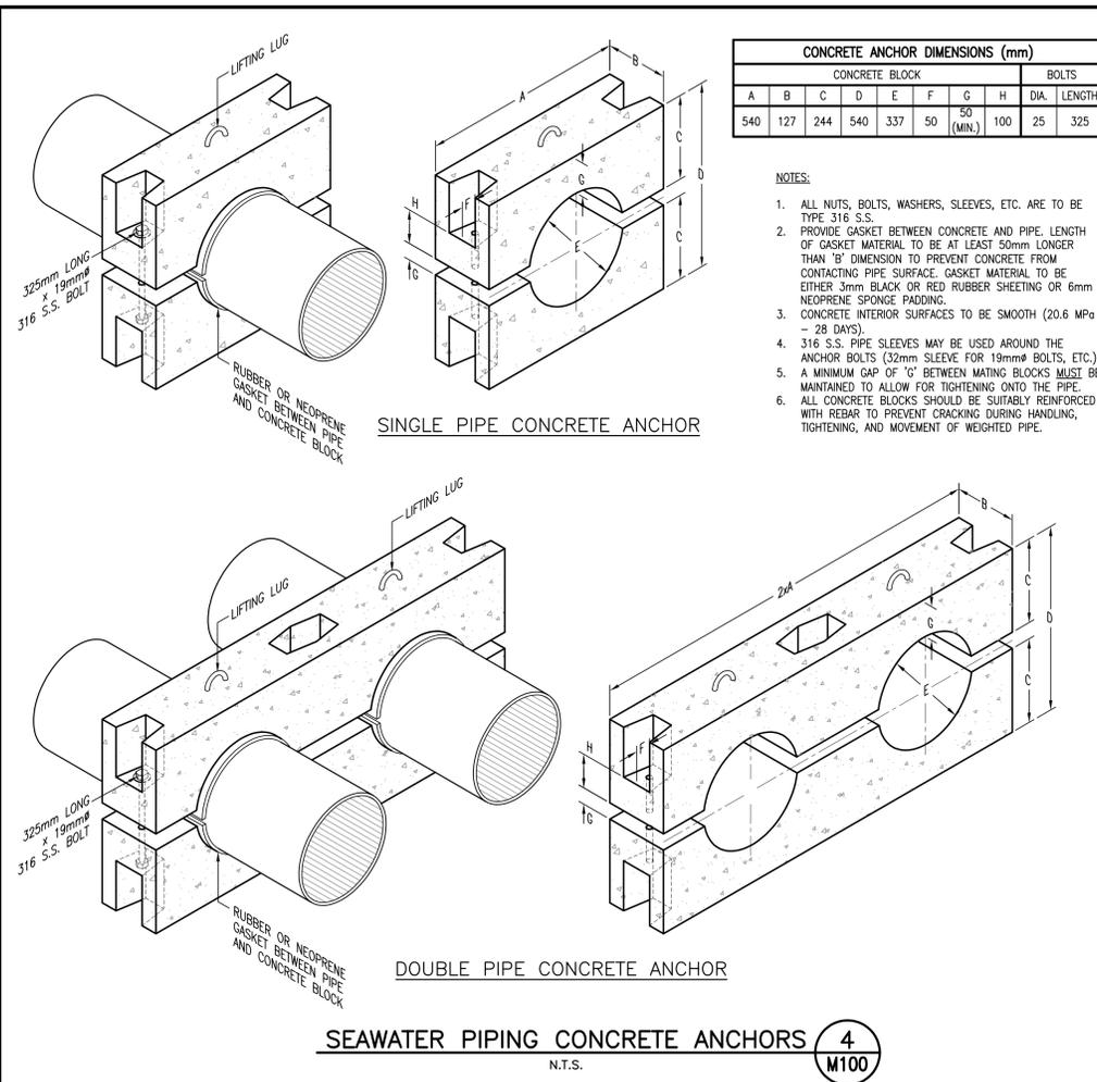
**SEAWATER PIPING CONCRETE ANCHORS 4**
