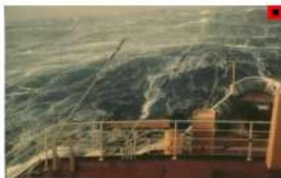
BEAUFORT FORCE 10 WIND SPEED: 48-55 KNOTS SEA: WAVE HEIGHT: 8-12.5M (26-41 FT), VERY HIGH WAVES WITH LONG OVERHANGING CRESTS, THE RESULTING FOAM, IN GREAT PATCHES, IS BLOWN IN DENSE WHITE STREAKS ALONG WIND DIRECTION, ON THE WHOLE, SEA SURFACE TAKES A WHITE APPEARANCE, TUMBLING OF THE SEA IS HEAVY AND SHOCK-LIKE, VISIBILITY AFFECTED
