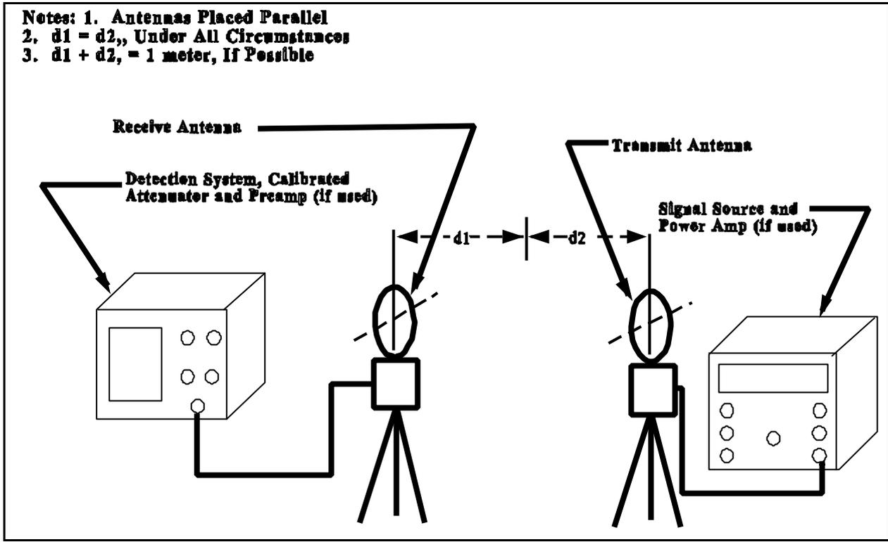
Figure 4 – Test Set-up for Magnetic Field Reference Measurement
