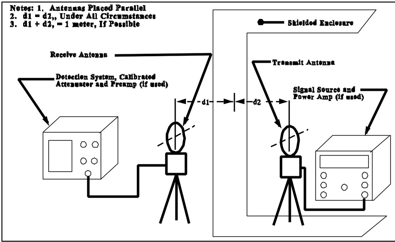
Figure 3 – Test Set-up for Magnetic Field Measurements
