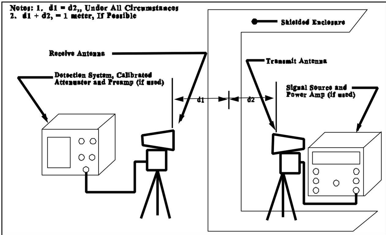
Figure 8 – Test Set-up for Plane-wave Measurement
