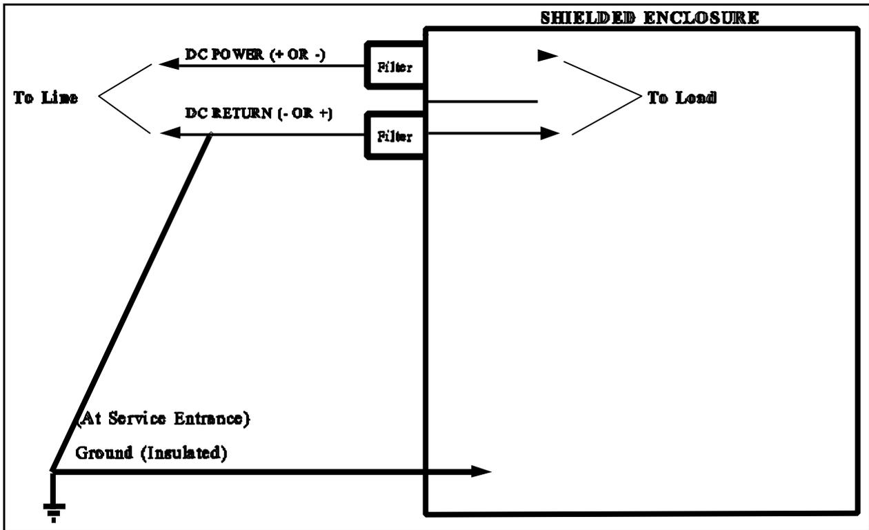
Figure 14 – Typical Power Line Configuration for DC Power
