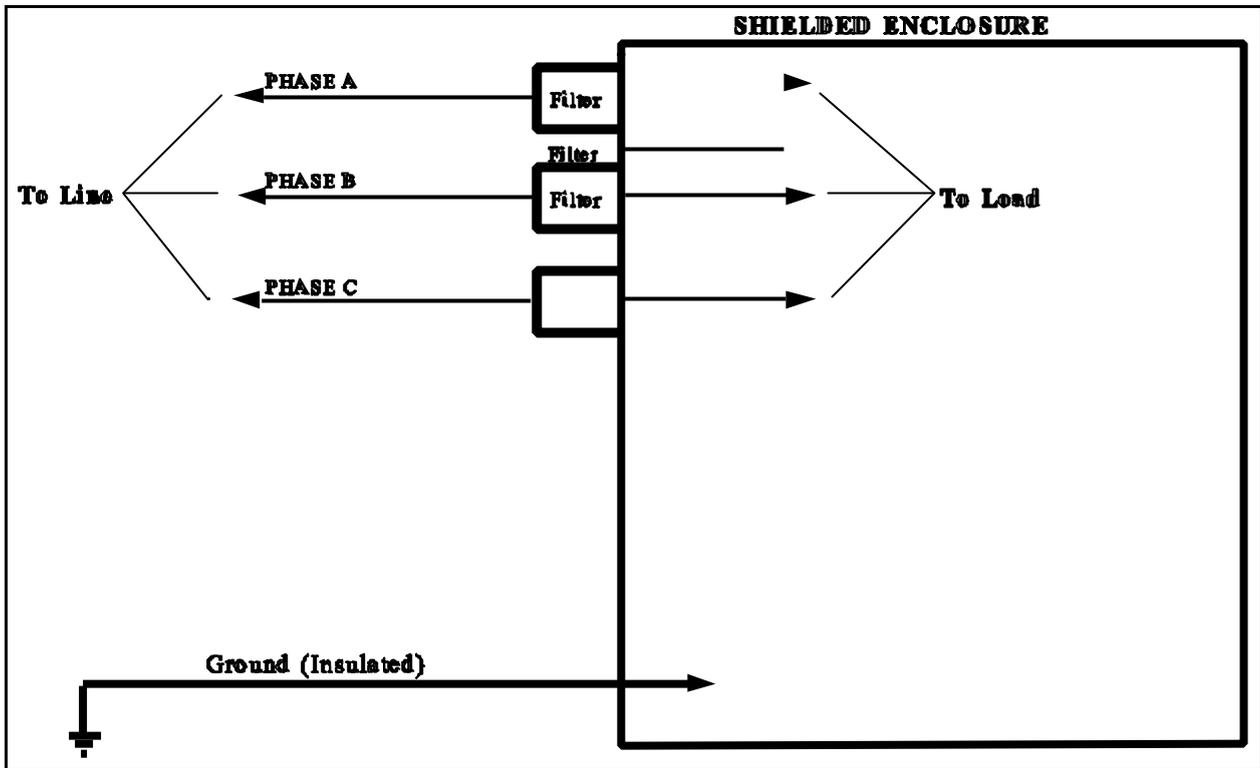
Figure 13 – Typical Power Line Configuration for 3 Phase, Delta
