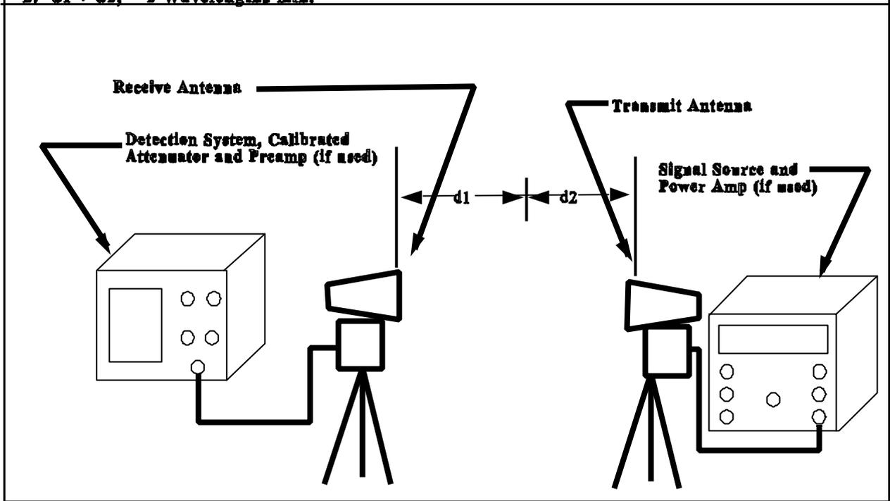
Figure 9 – Test Set-up for Plane-wave Reference Measurement
