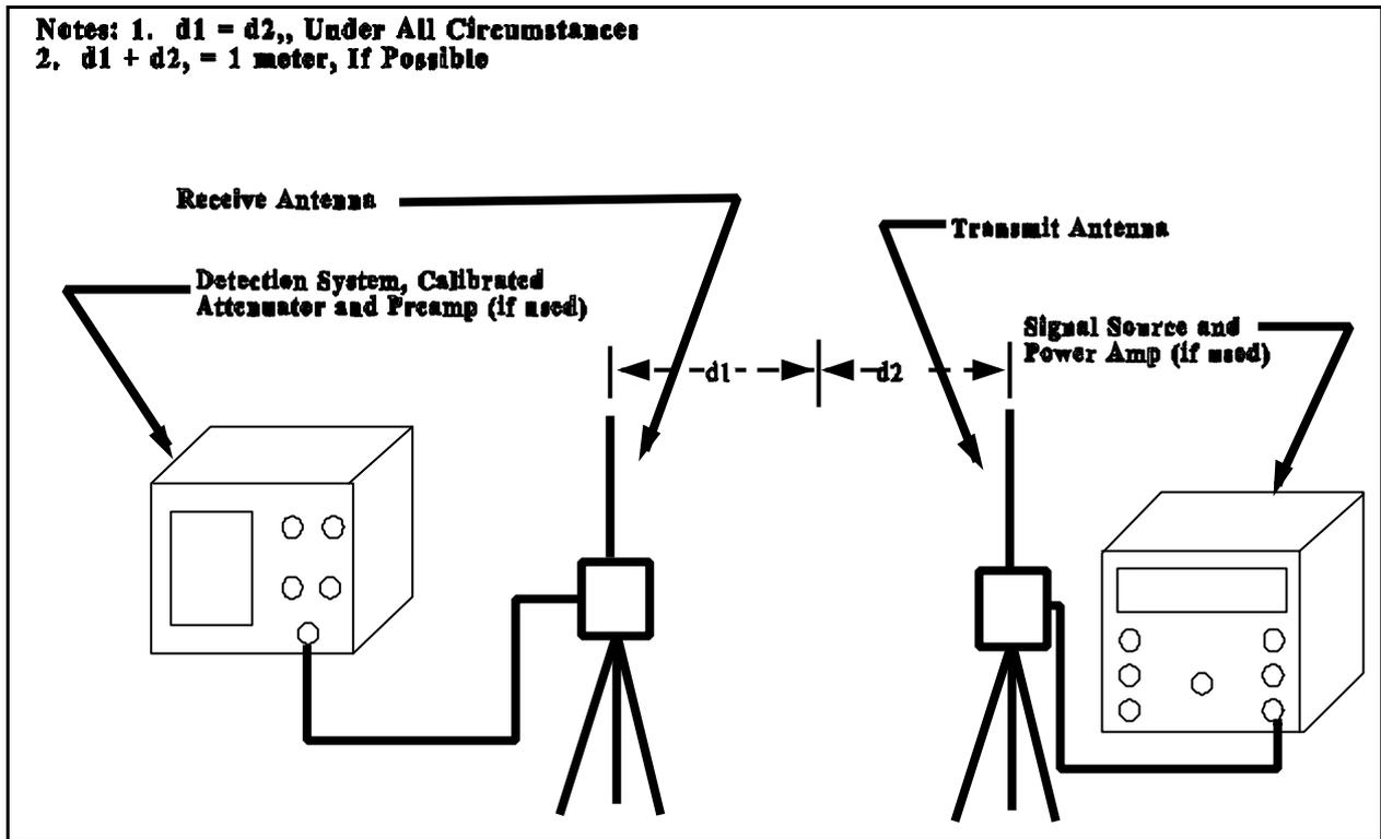
Figure 6 – Test Set-up for Electric Field Reference Measurement
