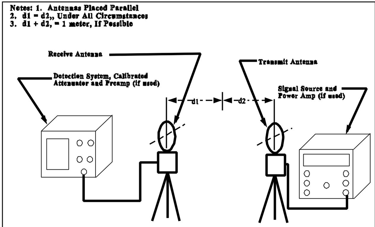
Figure 5 – Test Set-up for Electric Field Measurements
