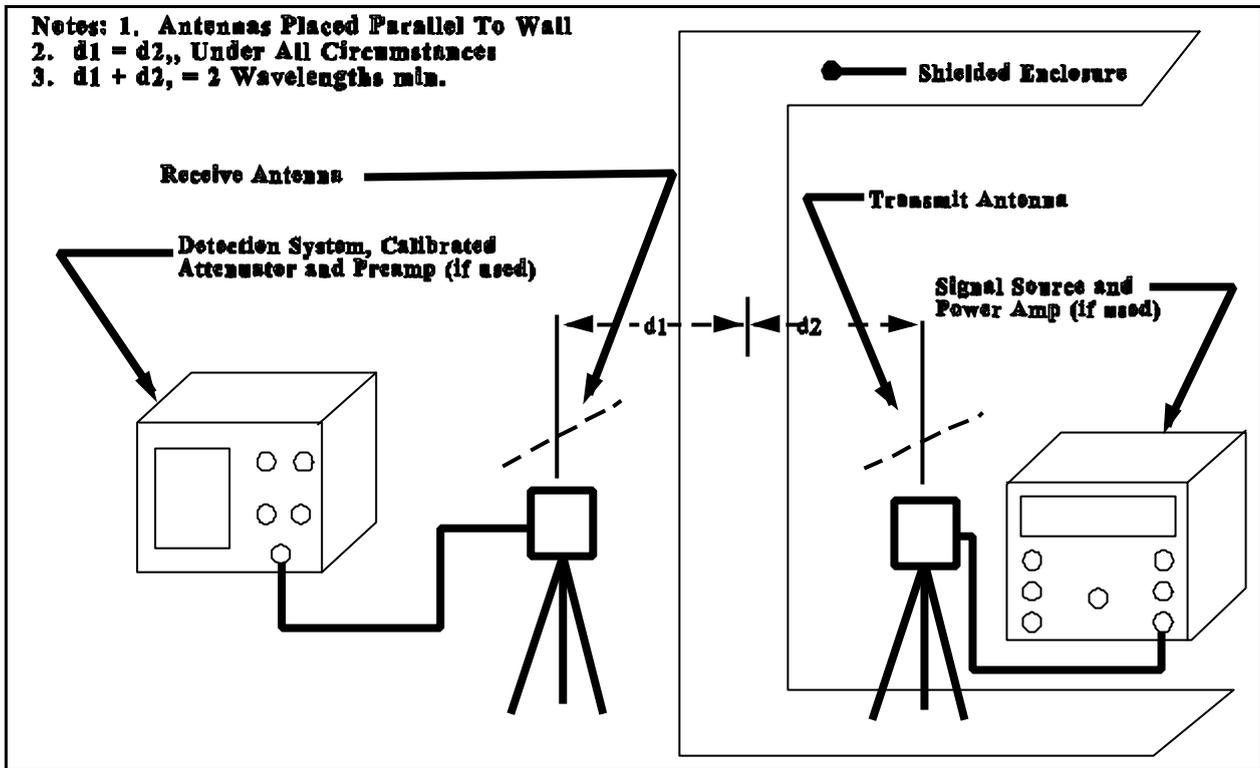
Figure 7 – Test Set-up for Plane-wave Measurement
