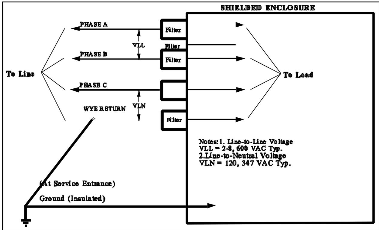
Figure 12 – Typical Power Line Configuration for 3 Phase, WYE
