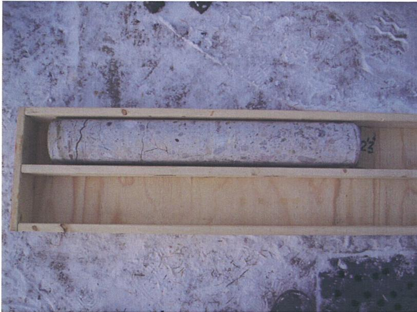
**Photo 3** – BH 05-4, RC 1 – 0'0" – 2'3" (wall thickness)
