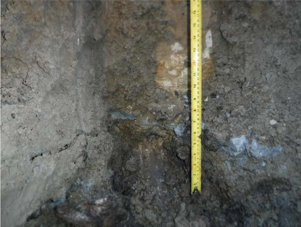
Test pit #1 – Layer of grout at bedrock
