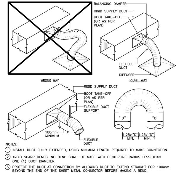
**FLEXIBLE DUCT INSTALLATION DETAIL**
