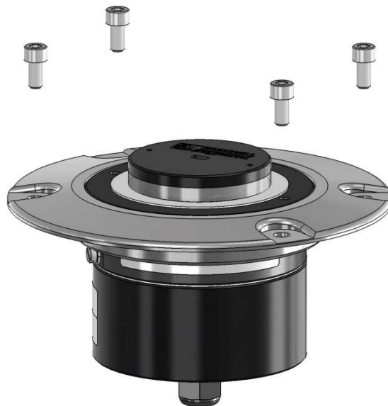
Figure 4 Mechanical attachment of recessed version
