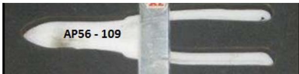
Photo 3 Etching of the tool's serial number will be in the tool cavity
