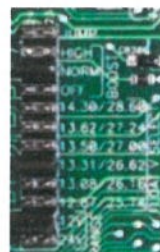
Field selectable jumper
