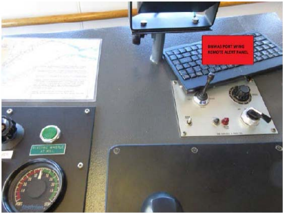
Port Wing Remote Alert Panel (RAP) Location
