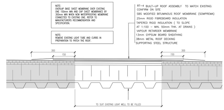
3 ROOF SECTION AT INFILL ROOF AT REMOVED LIGHT TUBES
