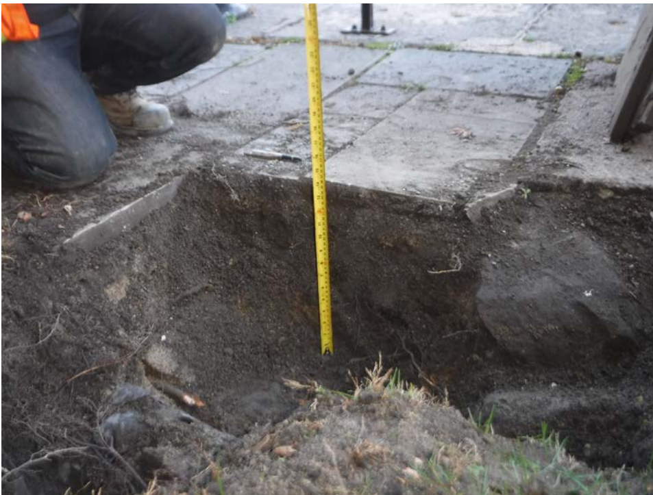
Test Pit #5 – Rubble behind wall to face of bedrock outcrop
