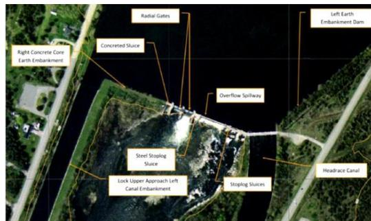
Scope: A comprehensive rehabilitation of the dam, lock and associated structures at Campbellford Dam 11 and Lock 13 are required including reconstruction of spillways, steel stoplog sluice, concrete repairs, rehabilitation of the left and right embankment earth dam and lock upper approach canal earth embankment and repair upstream and downstream lock concrete approaches.
