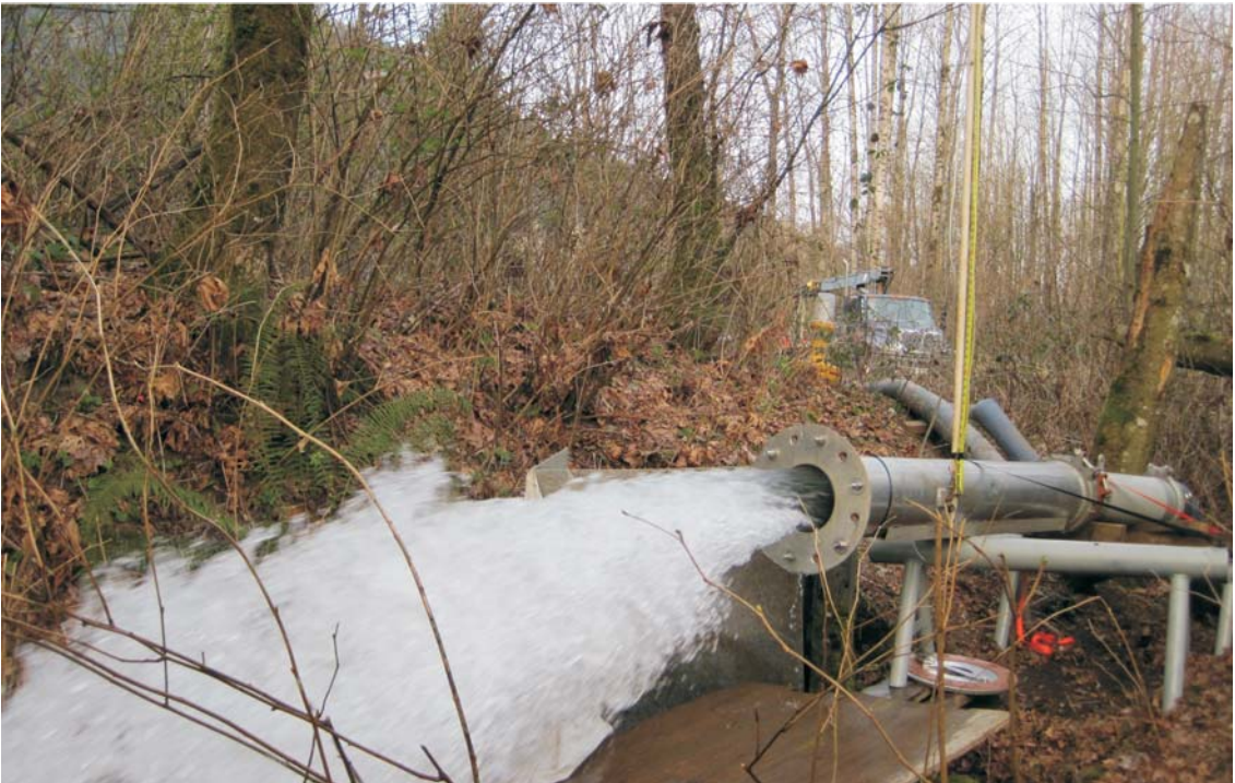
Photo 2. Orifice plate flow measurement device at discharge point during constant rate test ( Q = 139 \text{ L/s} [2,206 USgpm]).
