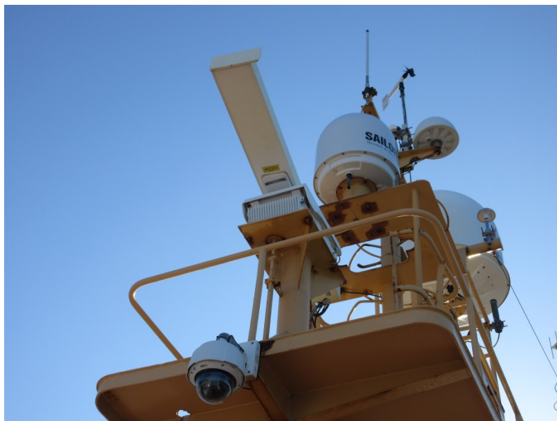
Picture: X-Band Turning Unit Location
