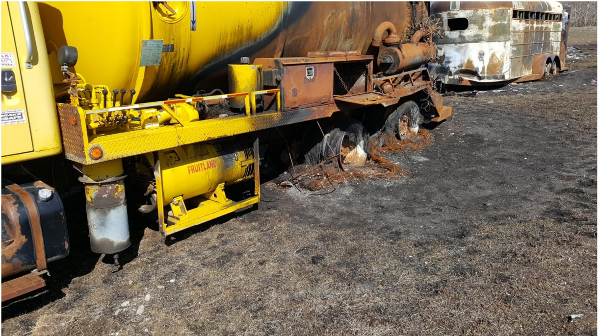
Photo 5g: Conditions of the vacuum truck after fire.
