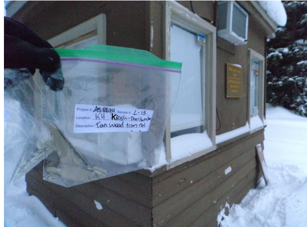
Photograph 14: Sample L-13 – Tan Painted Wood Trim on the Exterior of the Kiosk.
