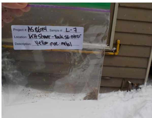
Photograph 09: Sample L-7 – Yellow Painted Metal Pipe on the South East Exterior Side of the Shower Building.
