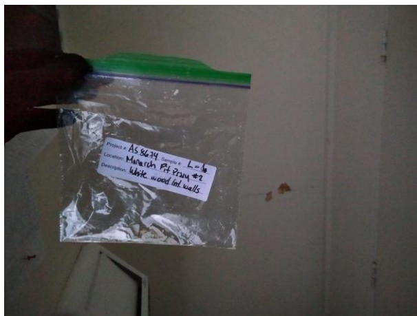
Photograph 04: Sample L-6 – Lead Containing White Paint on the Interior Wood Walls and Ceiling of Pit Privy #2.
