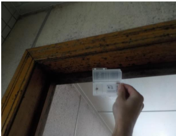
Photograph 15: Sample M-2 – Mould Tape Sample Collected from the Women's Bathroom Doorframe in the Shower Building.
