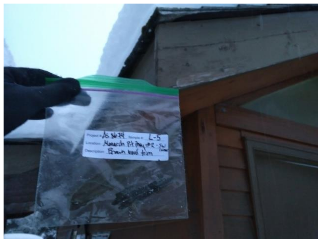
Photograph 03: Sample L-5 – Lead Containing Brown Paint from the Wooden Doors and Trim of Pit Privy #2.
