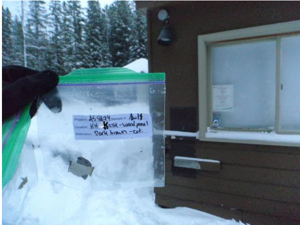
Photograph 13: Sample L-11 – Dark Brown Painted Wood Panels on the Exterior of the Kiosk.
