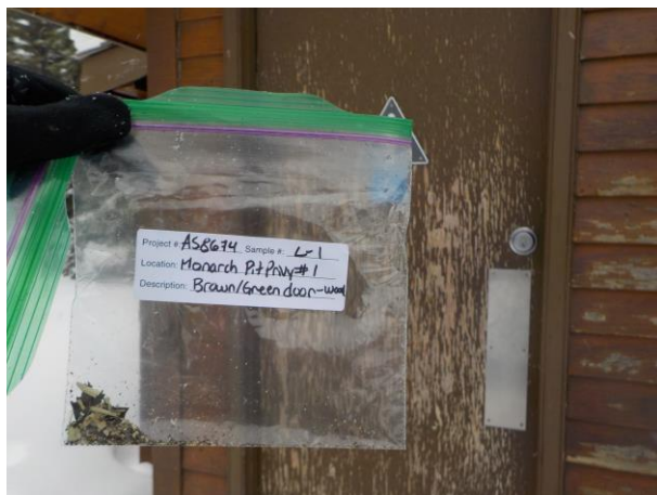
Photograph 01: Sample L-1 – Lead Containing Brown/Green Painted Wood Door and Roof Trim from the Pit Privy #1.
