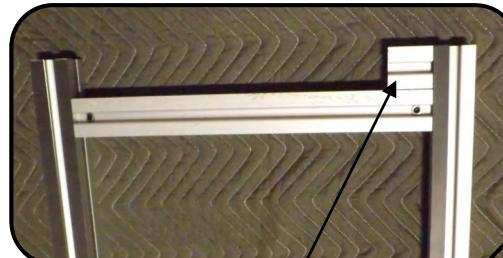
2" Spacer used on the top of each frame to position the cross rails accurately
