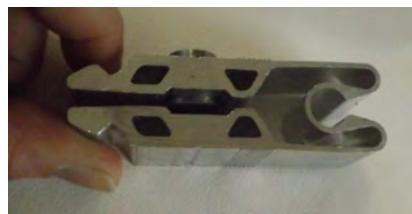
The clamp can be squeezed and inserted or removed from the aluminum framing at any time prior to tightening.
