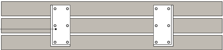
REFLECTED PLAN E-E: Fixings viewed from below
