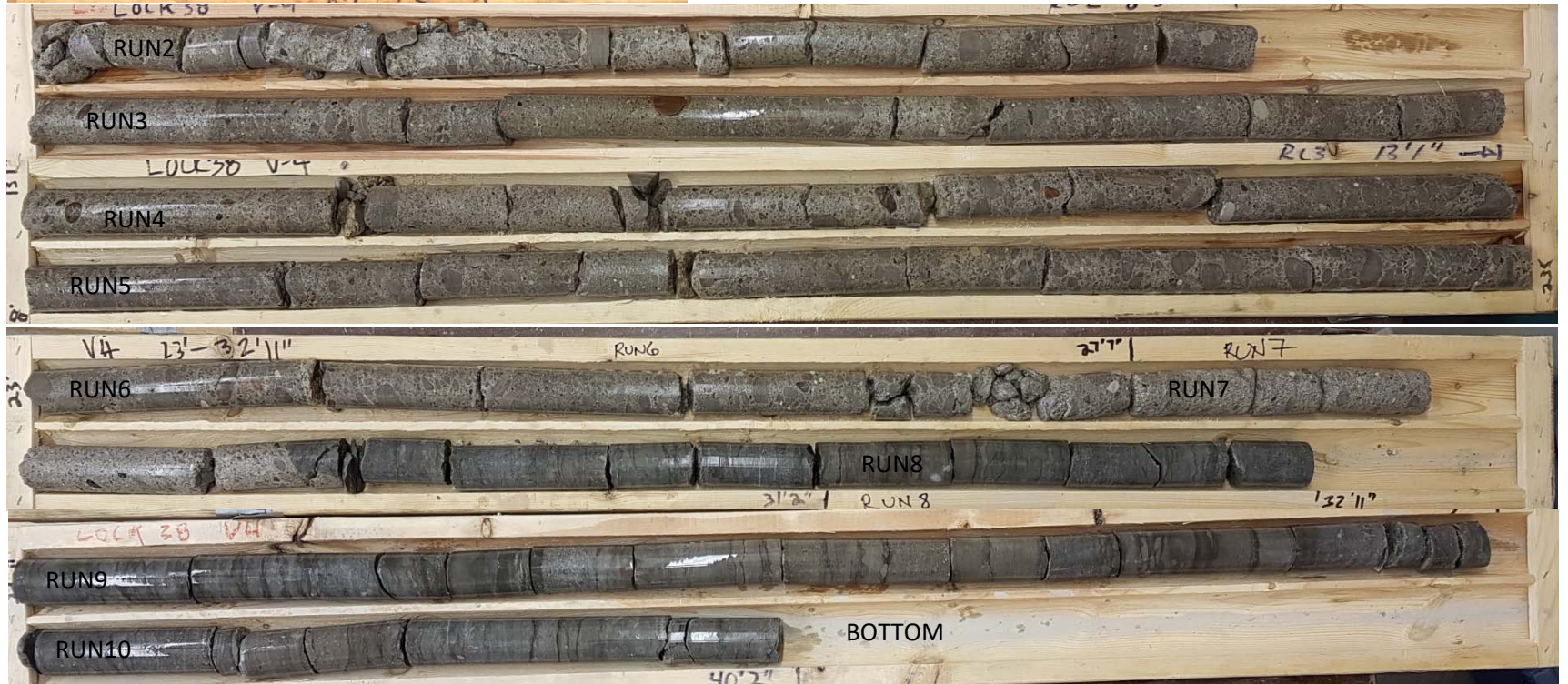
Photo of Concrete and Rock Cores from Borehole V-4.
