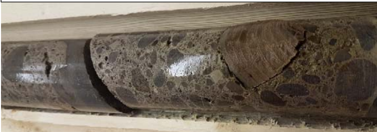
Wood encountered in concrete in Run 7.
