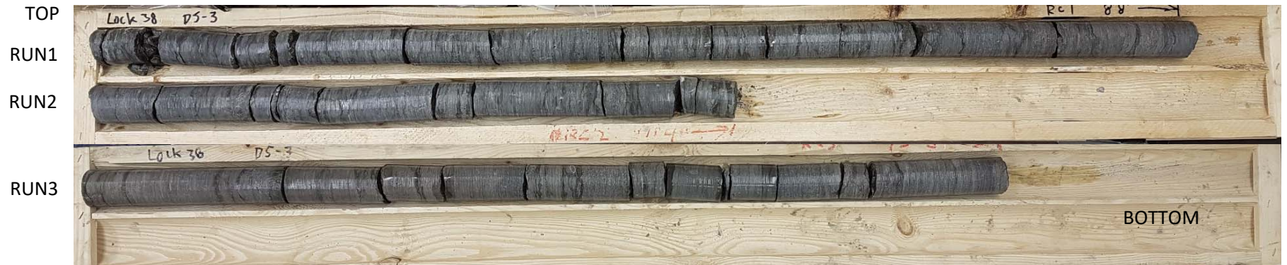
Photo of Rock Cores from Borehole DS-3.
