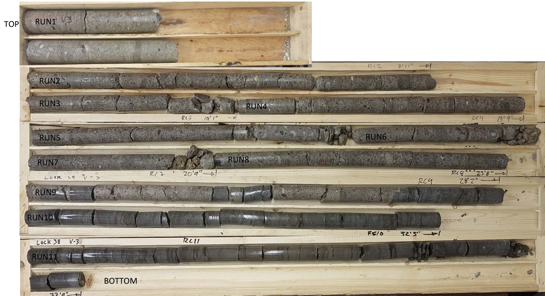
Photo of Concrete and Rock Cores from Borehole V-3.
