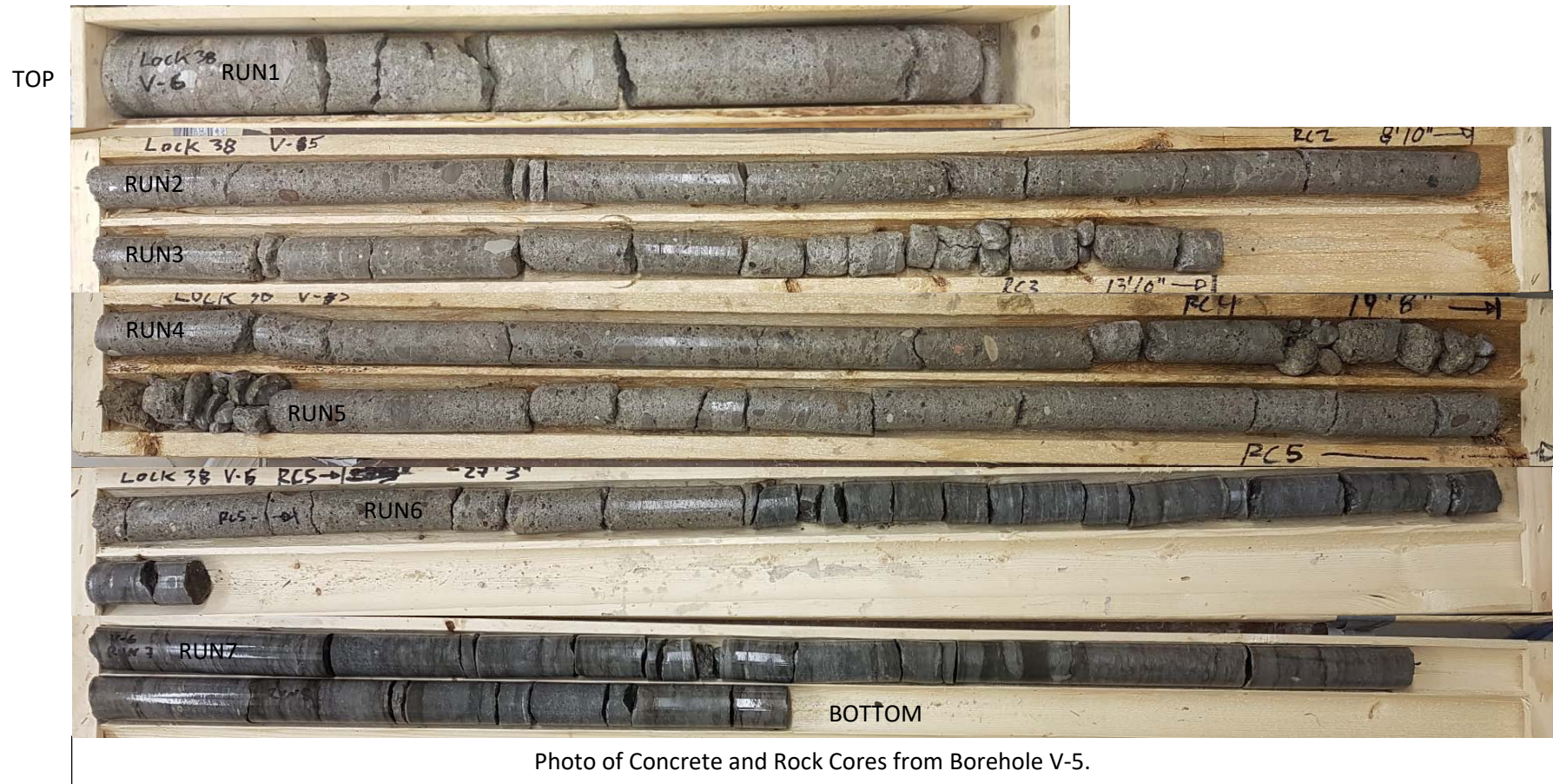
Wood encountered in concrete at top of Run 5.
