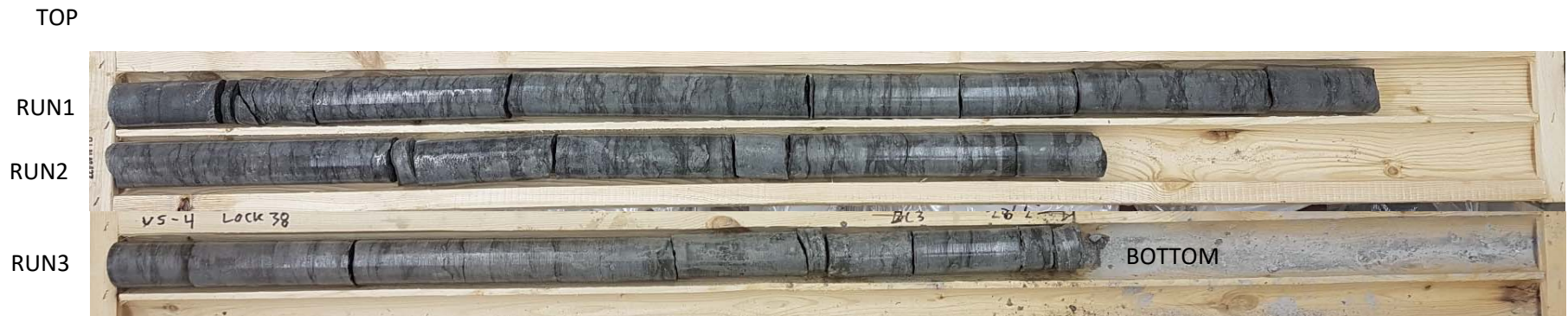
Photo of Rock Cores from Borehole US-3.
