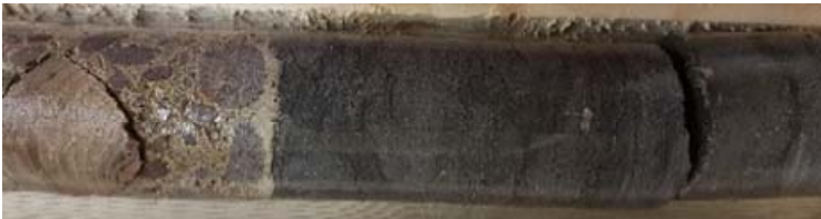
Bonded Concrete-Rock Interface.
