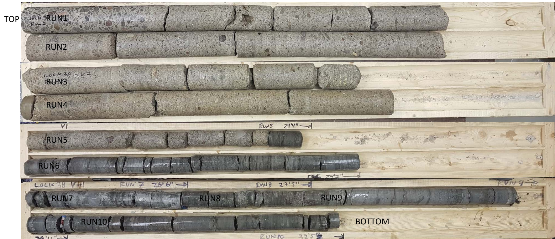
Photo of Concrete and Rock Cores from Borehole V-1.
