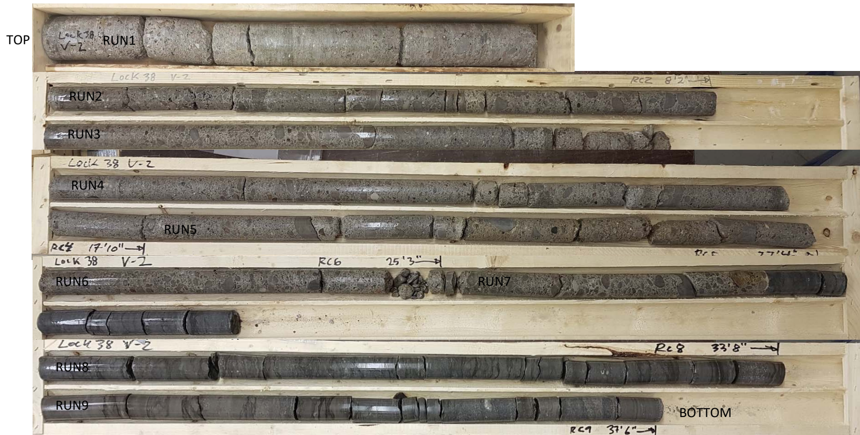
Photo of Concrete and Rock Cores from Borehole V-2.
