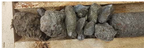
Wood encountered in concrete at top of Run 5.
