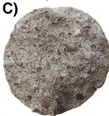
Coring Fracture at base
