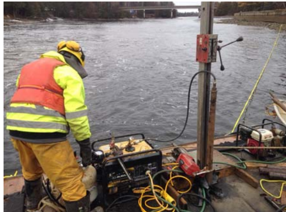
Portable coring on raft.
