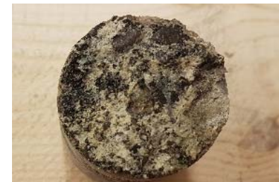
White and black staining at concrete joint.
