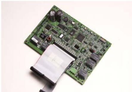
Figure O-GI-2. Tracer AH540 Control Board
