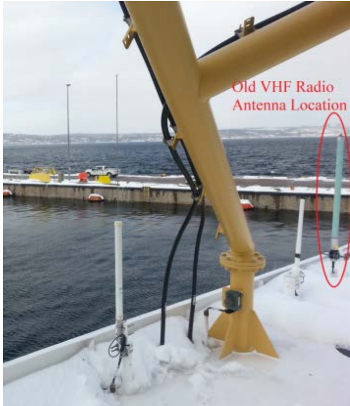
Photo #2 – Old VHF Radio Antenna Location
