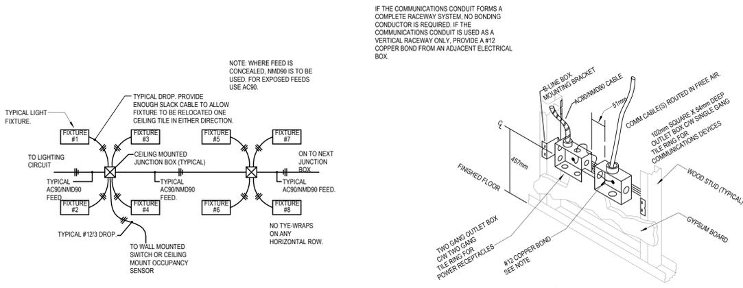
IF THE COMMUNICATIONS CONDUIT FORMS A COMPLETE RACEWAY SYSTEM, NO BONDING CONDUCTOR IS REQUIRED. IF THE COMMUNICATIONS CONDUIT IS USED AS A VERTICAL RACEWAY ONLY, PROVIDE A #12 COPPER BOND FROM AN ADJACENT ELECTRICAL BOX.
