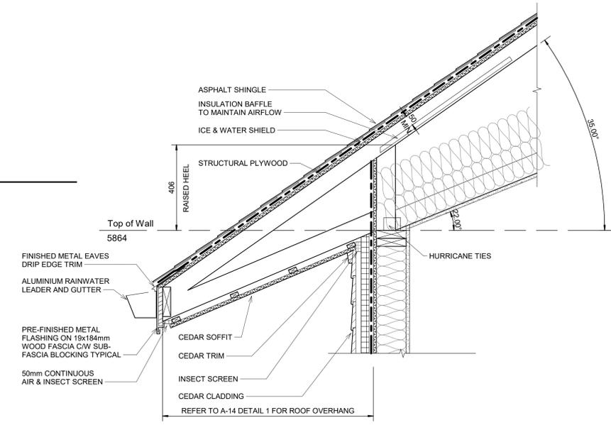
5 SECTION AT SLOPED CEILING
