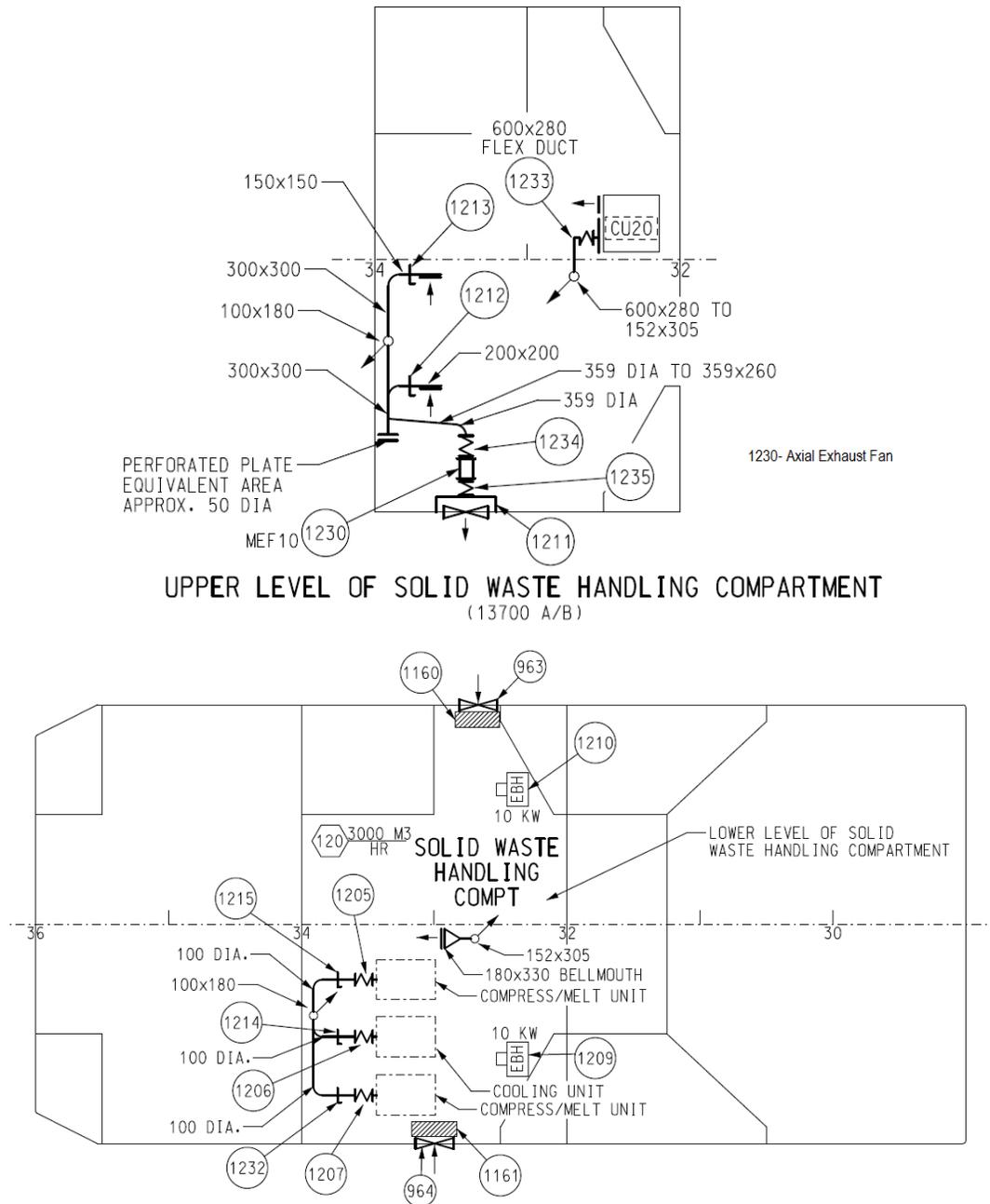
Figure 1- Ventilation Details Upper (Mezzanine) and Lower Level Solid Waste Handling Compartment
