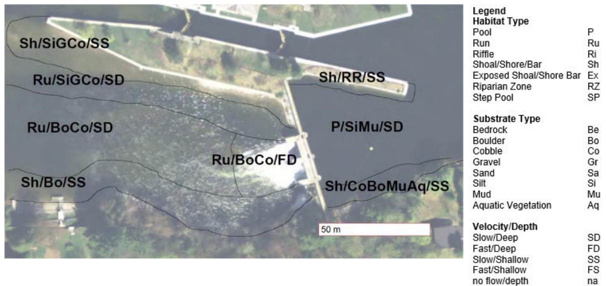
Figure 7. Diagram of site depicting substrates/velocities and depths as relating to fish habitat (Arcadis 2017)
