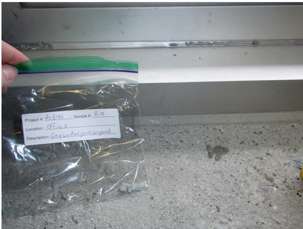
Photograph 02: Sample A17 - Asbestos-Containing Grey Window Joint Compound – Office 6
