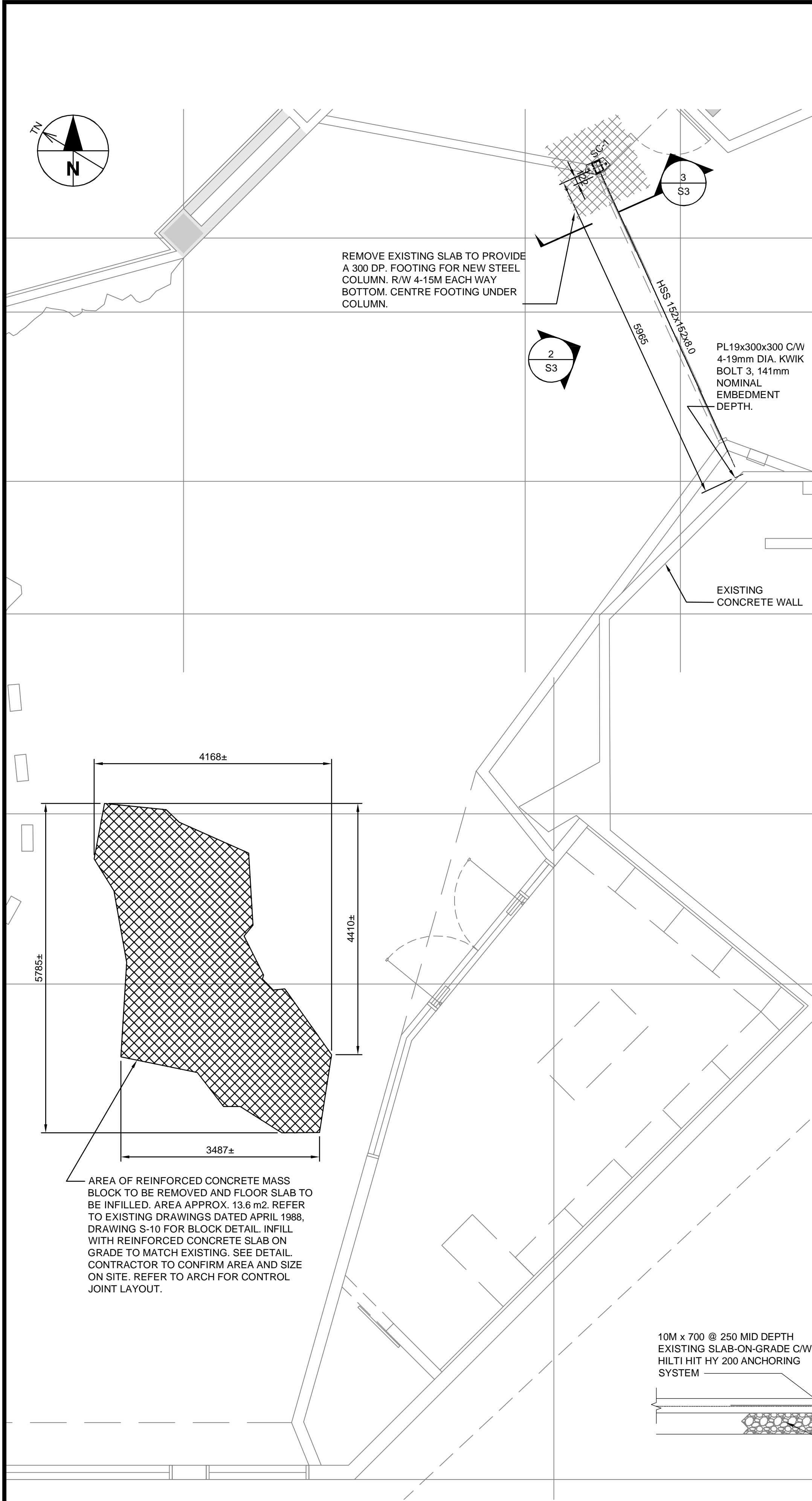
1 | NEW WALL OPENINGS & SLAB INFILL PARTIAL PLAN S3 1:50
