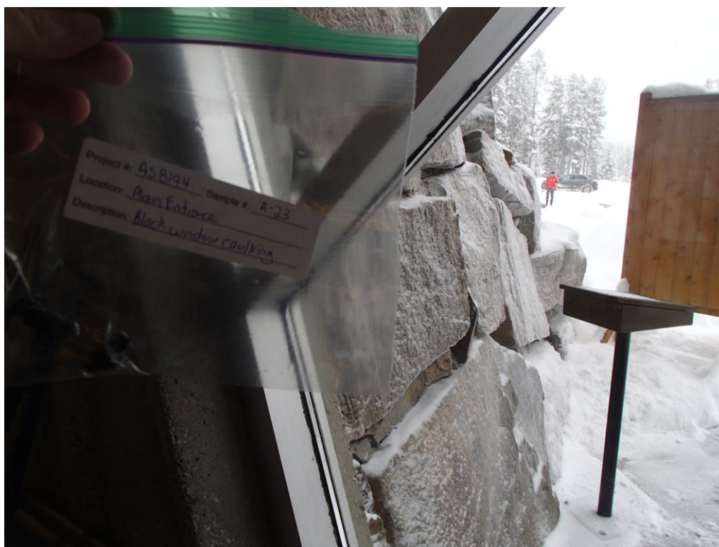
Photograph 04: Sample A23 - Asbestos-Containing Black Window Caulking – Interior of Main Entrance
