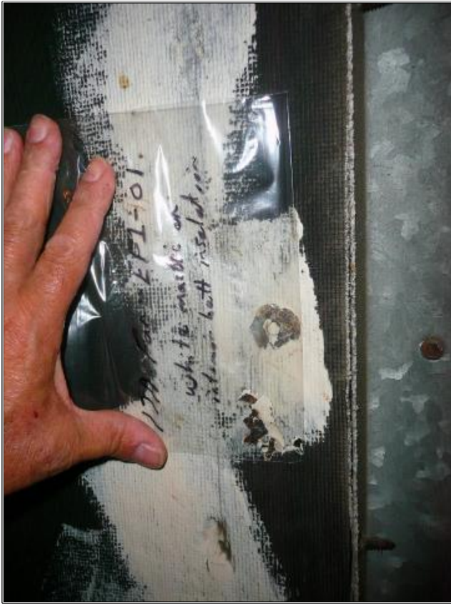
The White and Black Mastics on Interior Batt Insulation as observed and sampled within the Exhaust Fan EFl in the Main Fan Room was found to be None Detected for asbestos.
