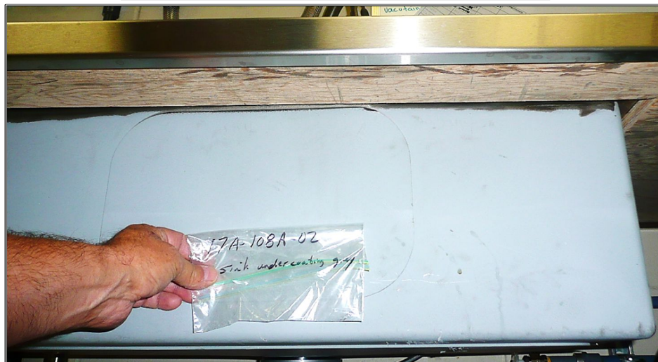
Sinks with White, Off-White and Light Grey Undercoating as sampled were found to be None Detect for asbestos.
