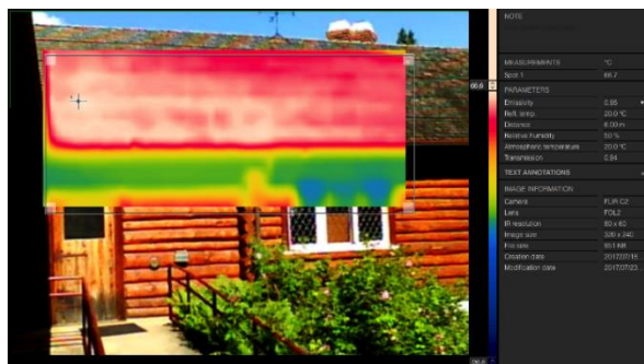
Figure 4: West Facing Roof (max temp 66.7°C)
