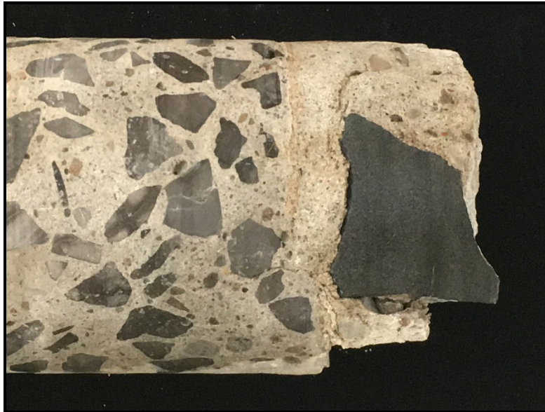
Core F3. A different concrete is seen on the inner side of the core. The large aggregate on far right has a size of 30 to 60 mm
