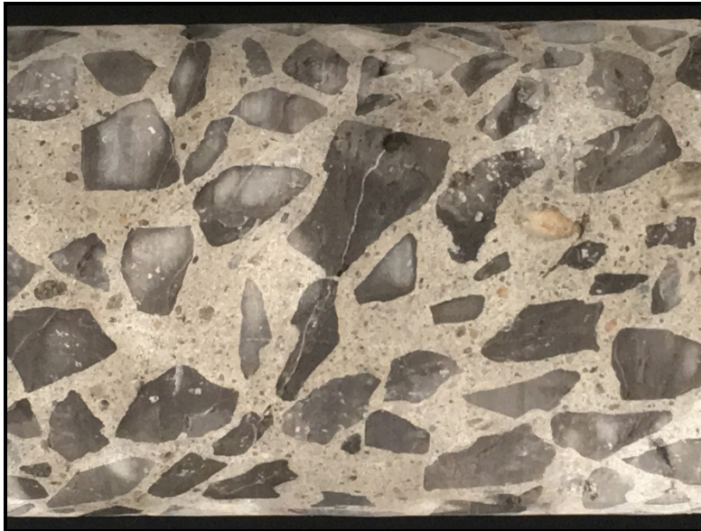
Core F2. Close-up view of aggregates. Silica gel and cracks are visible through the aggregates and cement paste
