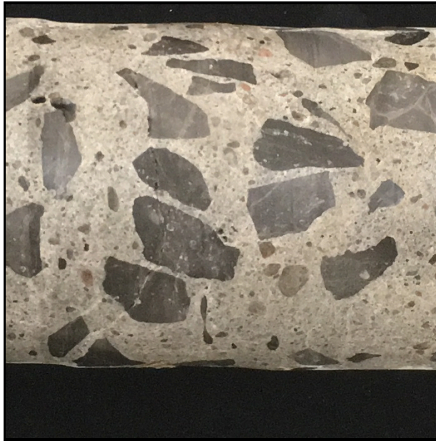
Core F5. Close-up view of the core with cracks passing through the aggregates
