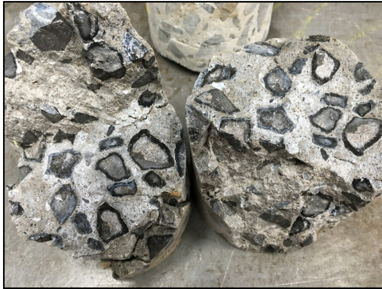
Core F4. After the compression break. Rings around the aggregates are clearly visible.
