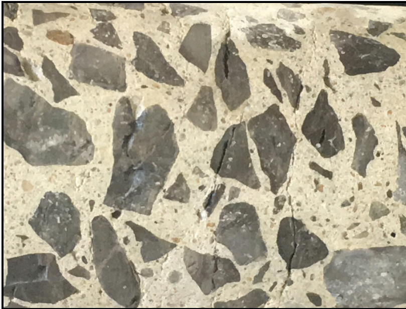
Core F6. Several cracks passing through the aggregates
