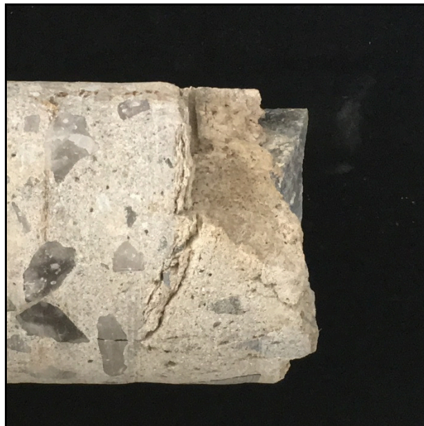
Core F3. Concrete delamination
