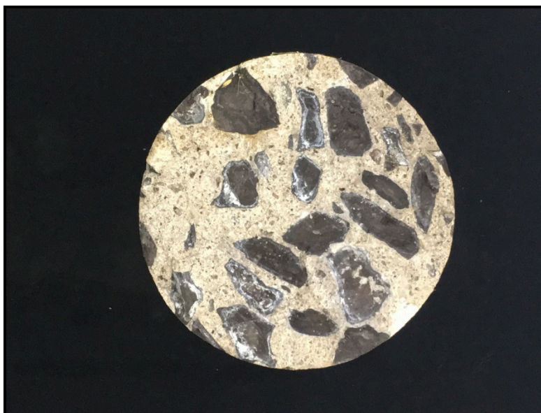
Core F8. Silica gel around the aggregates
