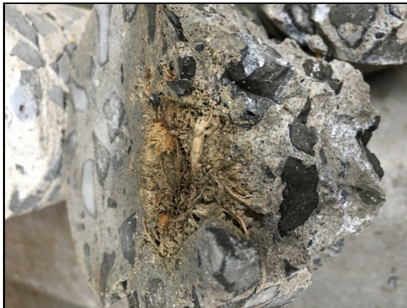
Core F4. After the compression break, wood is clearly visible in the concrete.
