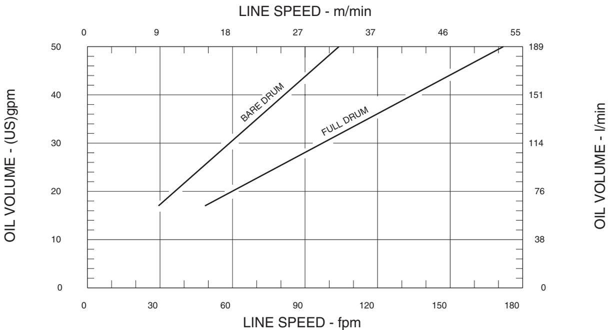
Performance graphs are based on standard hydraulic motor, gear ratio and cable drum with 5/8 inch diameter wire rope.
