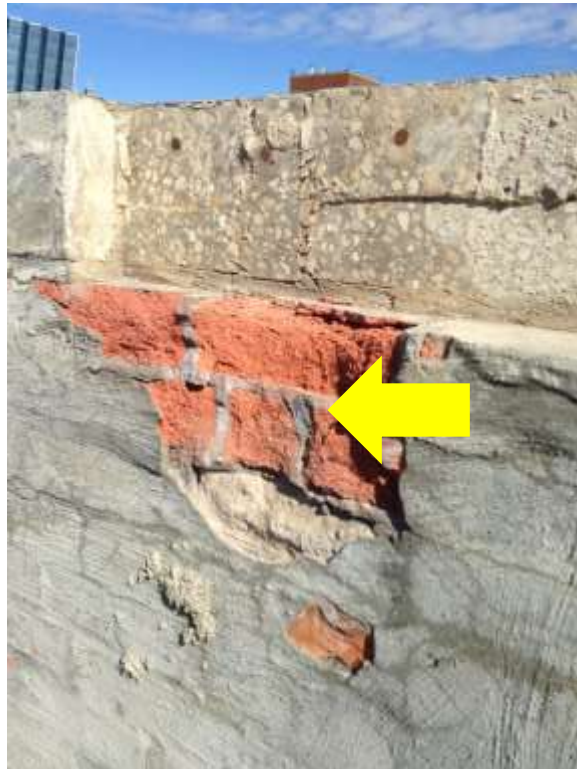
Asbestos Mortar, (Sample S0018), Roof (Location:36)
