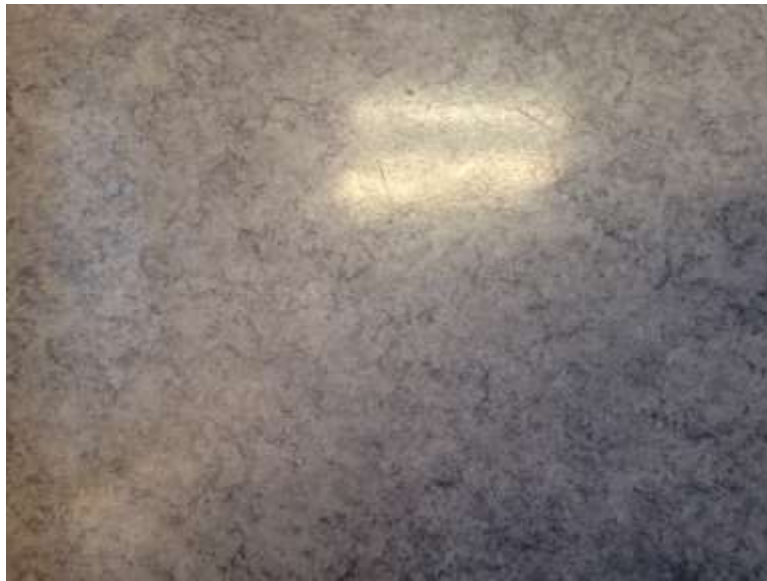
Non-asbestos Vinyl Sheet Flooring, Blue, (Sample S0005), 1-116 (Location:3)
