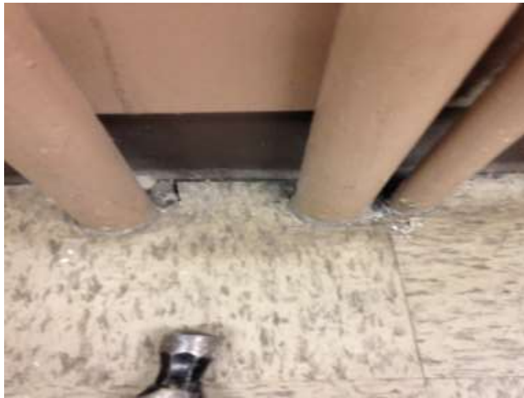
Non-asbestos Vinyl Floor Tiles, 12X12 Light Brown with Grey Flecks (Sample S0001), 4-114 (Location:1)
