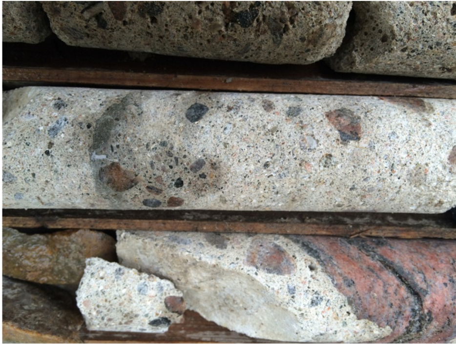
DH15-2 Box 1 of 2: Detail of concrete with rounded to angular particles and granitic type aggregate material.
