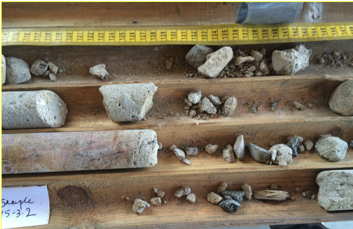
DH15-3 Box 1 Detail showing iron weathering within concrete core.
