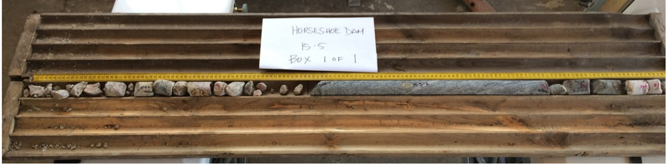
DH15-5 Box 1 of 1: concrete core at the top left and bedrock on the right of box.
