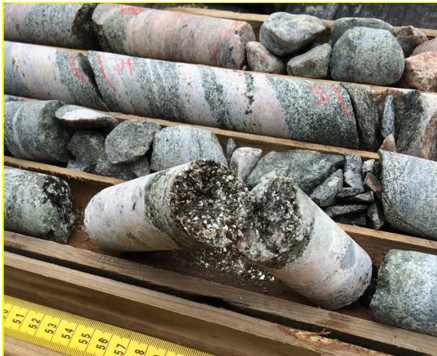
DH15-1 Box 2 of 2 showing detail of biotite seam
