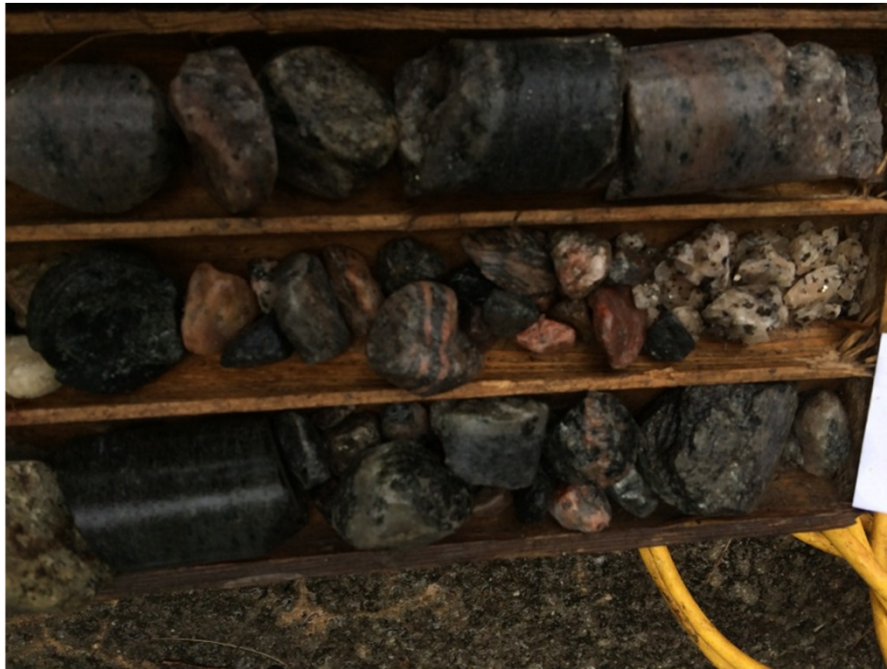
DH15-2 Box 2 of 2: Detail of gouge zone in rock. Rounded to angular rock fragments of small size.
