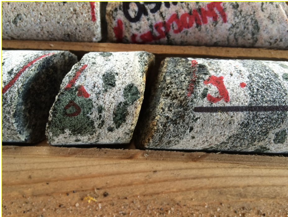
DH15-8 detail showing large chlorite crystals and chlorite foliation/alteration.
