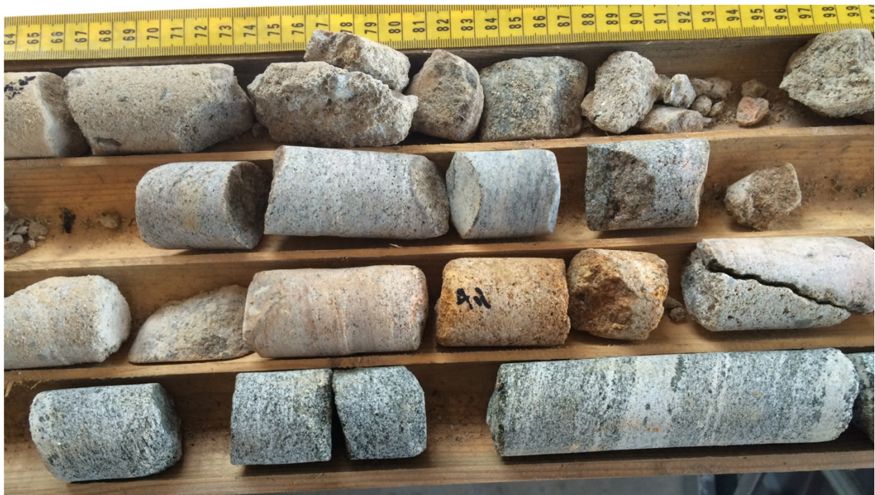
DH15-3 Box 1 Detail showing iron weathering within concrete core.
