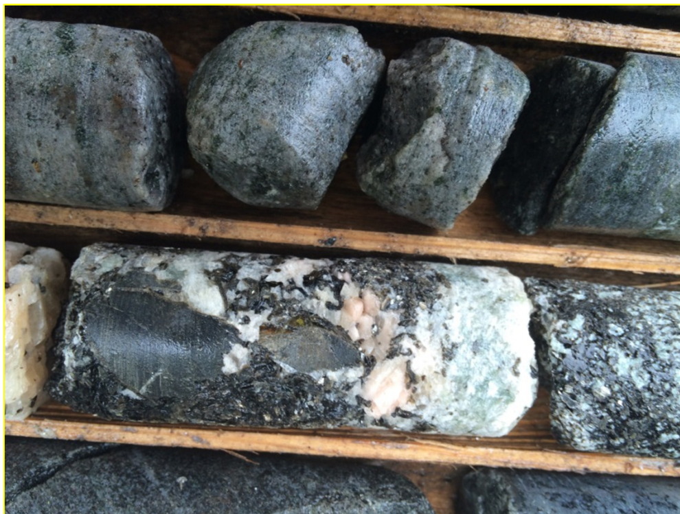
DH15-2 Box 2 of 2. Detail of large biotite crystals with no preferred orientation.
