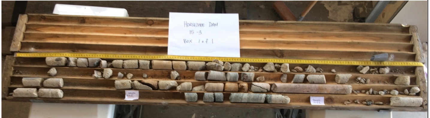
DH15-3 Box 1 of 1. Concrete core showing poor recovery of core.
