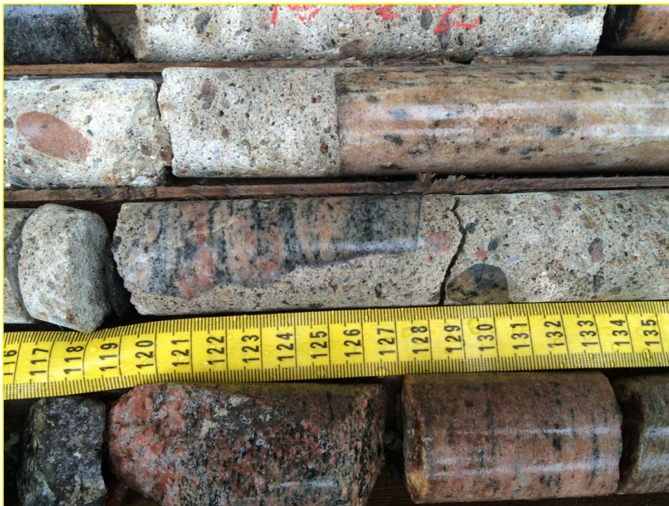
DH15-2 Box 1 of 2: Detail of aggregate material and concrete.
