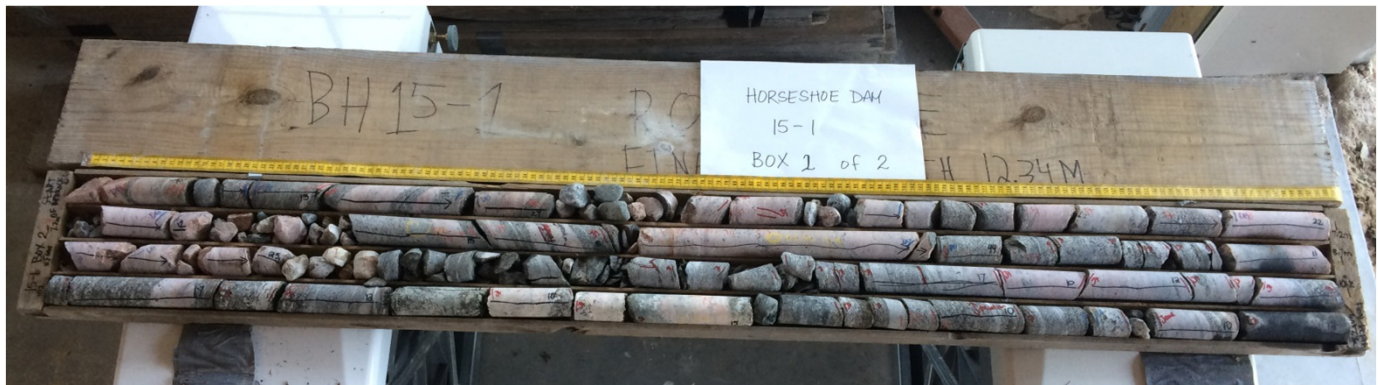
DH15-1 Box 2 of 2 showing rock core from 5.7 m to 11.7 m. Feldspathic rich layered intrusive of moderate metamorphism with gneissic texture at 45 degrees to core axis. Medium to coarse grained with poorly defined foliation.
