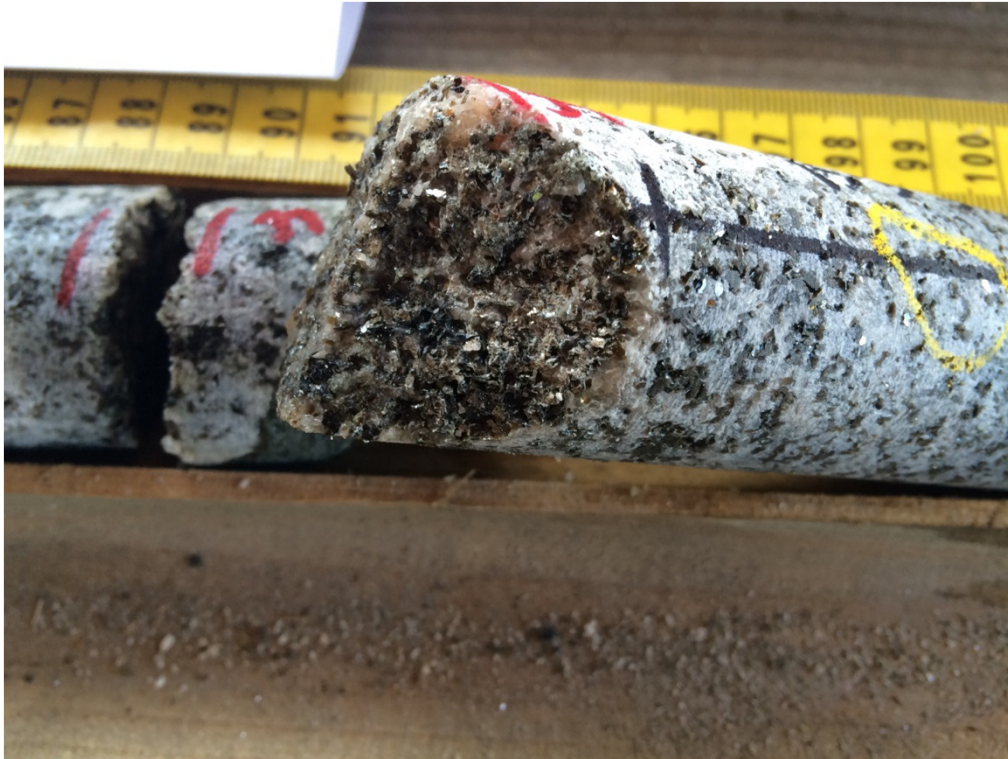
DH15-8 detail showing biotite foliation at 1.21 from hole collar
