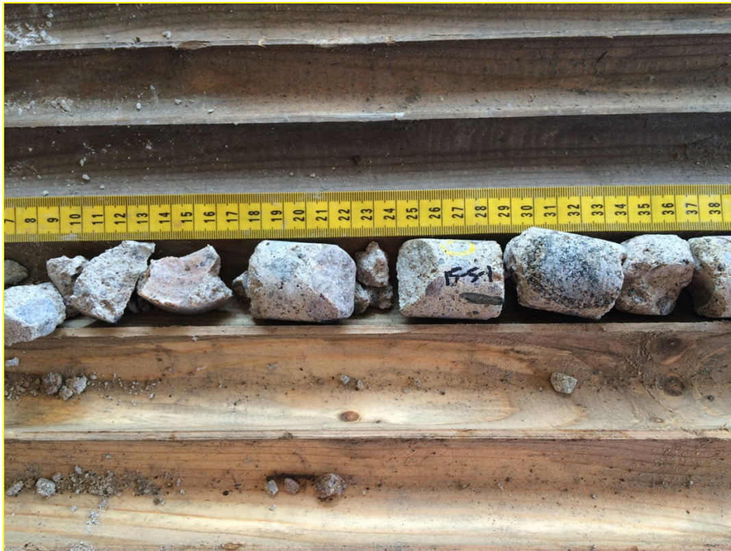
DH15-4 detail showing poor concrete and small sample size of sample 15-5-1.
