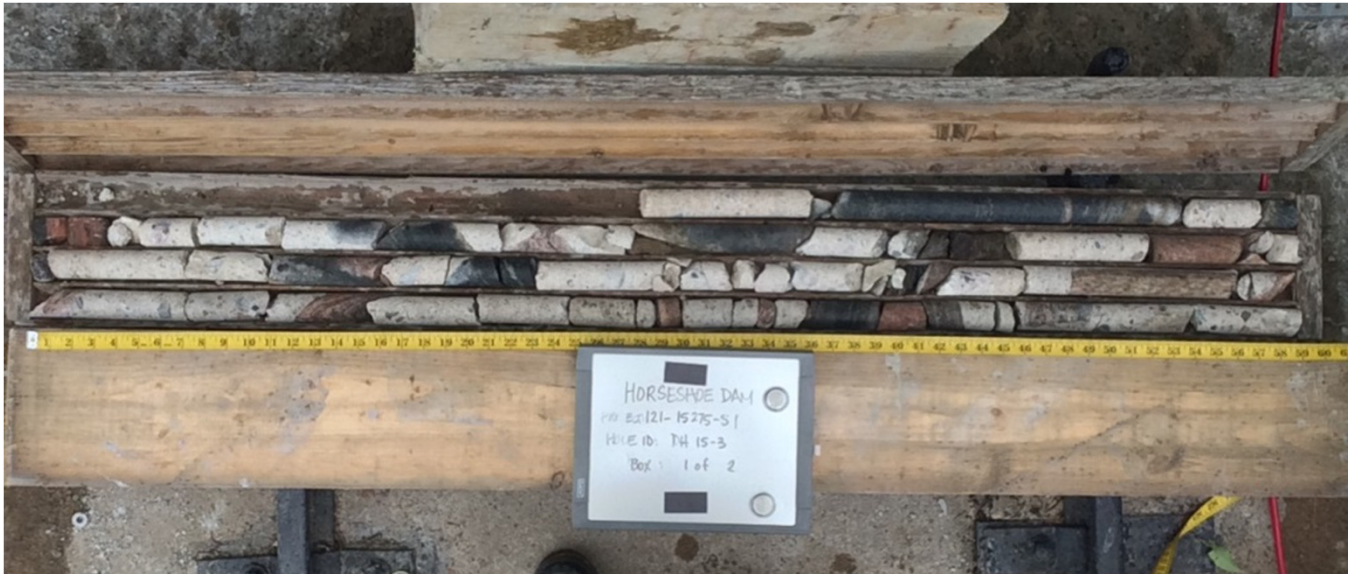
DH15-2 Box 1 of 2: Showing concrete from hole collar to 8.3 m. First 71 cm of core no retrieval due to highly weathered concrete.
