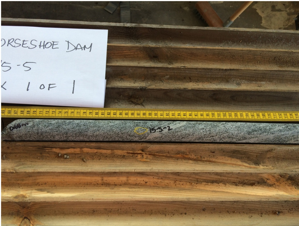
DH15-5 Box 1 of 1: detail of bedrock section of very good rock quality. Sample 15-5-2.
