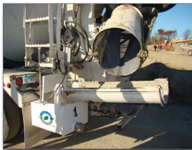
Figure 7. Chute washout box
