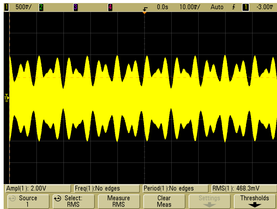
Figure 4 - MSK DGPS Signal + R-Mode Signal (CW1 and CW2) at 10 ms timescale
