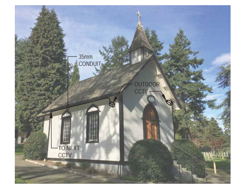
4 CHAPEL CCTV ELEVATION E1.00 NOT TO SCALE
