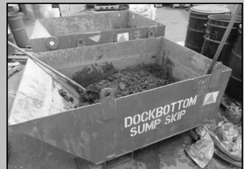
ADEQUATE waste grit storage.
