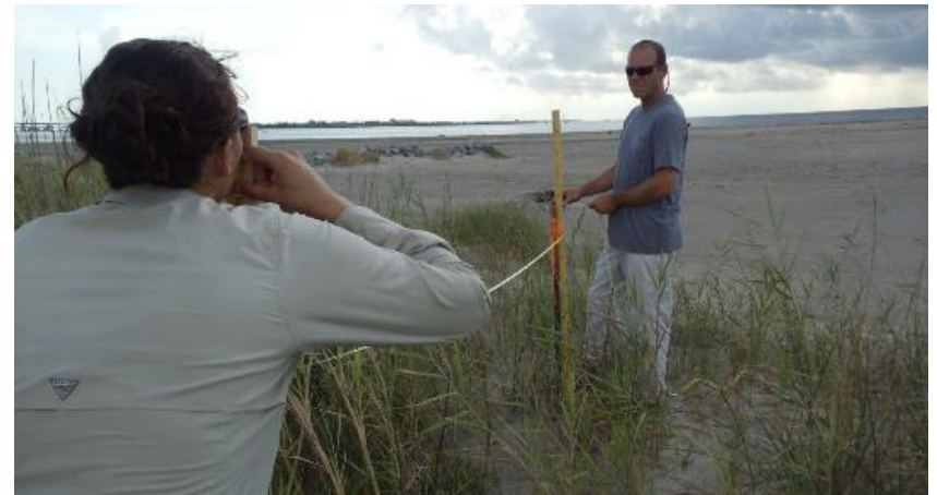
Figure 6.5 Beach profiling using the pole and horizon method
