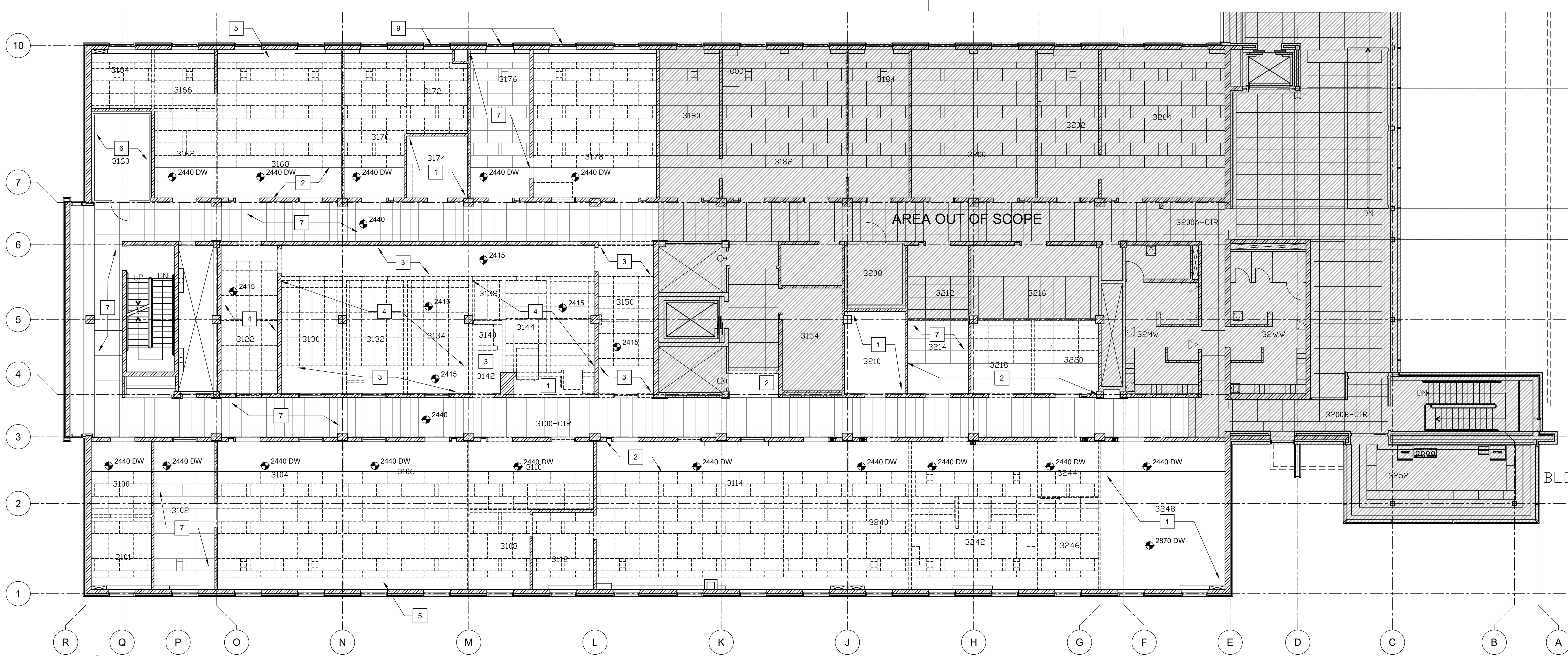
1 3RD FLOOR REFLECTED CEILING PLAN - DEMOLITION SCALE 1:100
