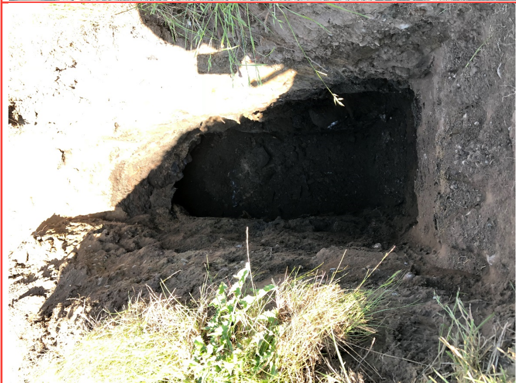
Photo 4: TP18-02 terminated at 2.9m in bedrock
