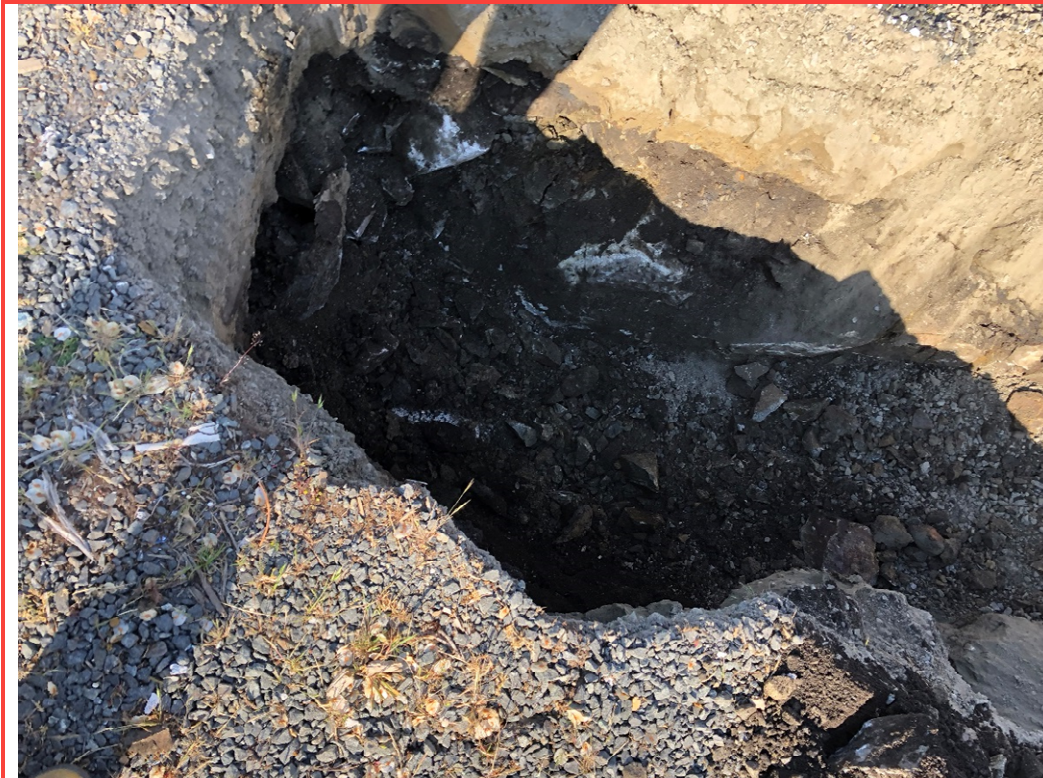
Photo 3: TP18-01 terminated at 1.2m in bedrock
