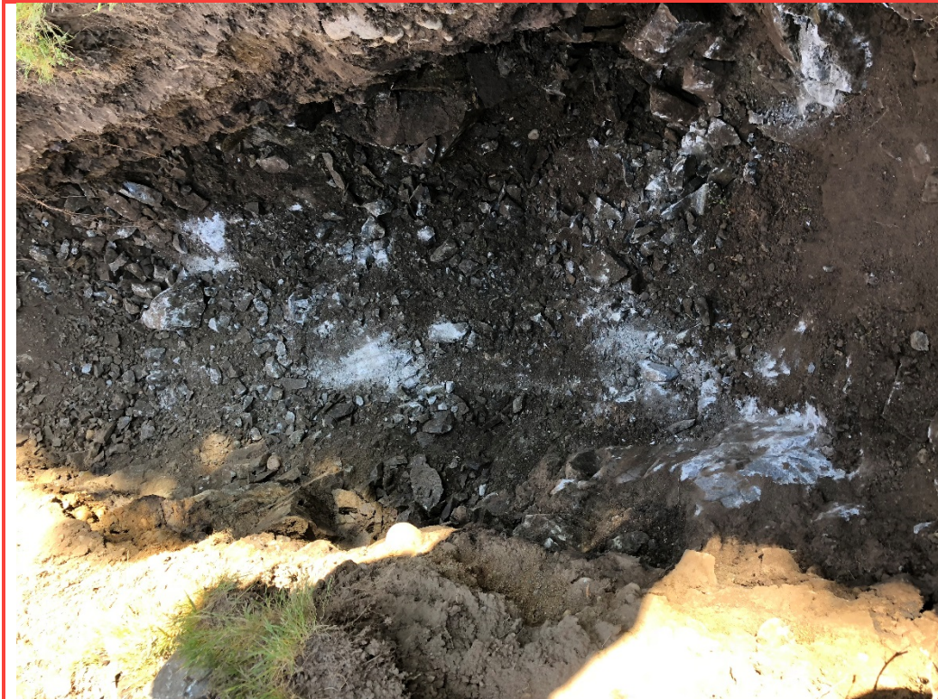
Photo 5: TP18-03 terminated at 1.3m in bedrock
