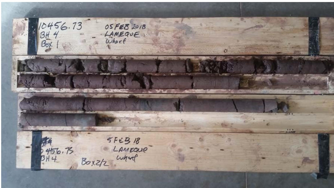
Mudstone bedrock extracted from BH18-04. 6.4 to 10.4 metres below existing top of deck.
