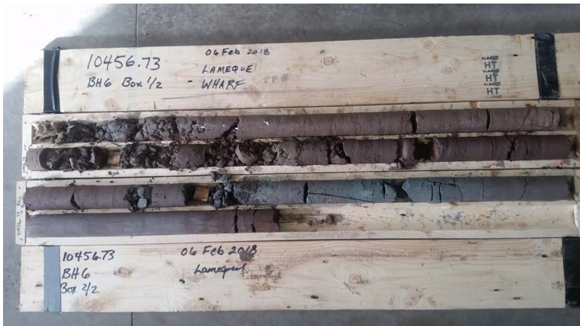
Mudstone bedrock extracted from BH18-06. 8.1 to 12.4 metres below existing top of deck.
