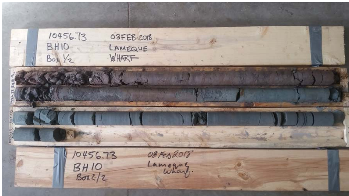
Bedrock extracted from BH18-10. Mudstone: 14.0 to 16.7 metres below existing top of deck. Sandstone: 16.7 to 18.4 metres below existing top of deck.
