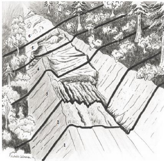
Figure 15: Recontouring Steps for Road/Trail Corridor
