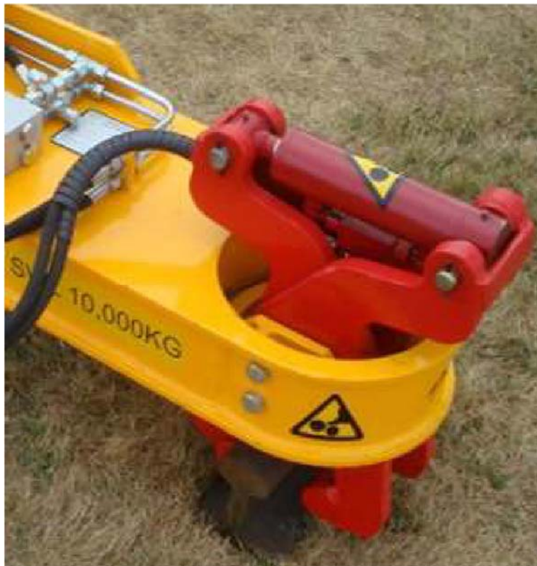
Figure 23: Example of a hydraulic clamp
