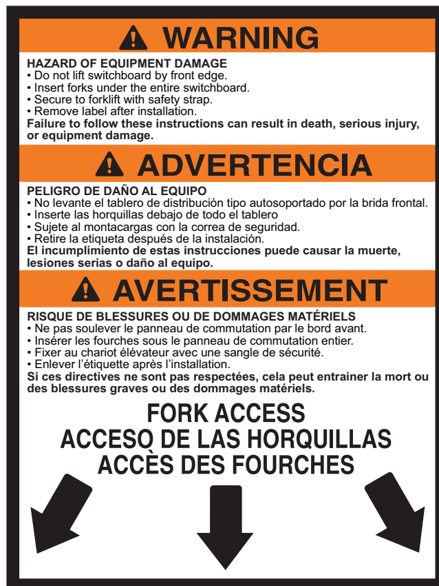
Figure 2 – Warning Label, Rainproof Switchboards
