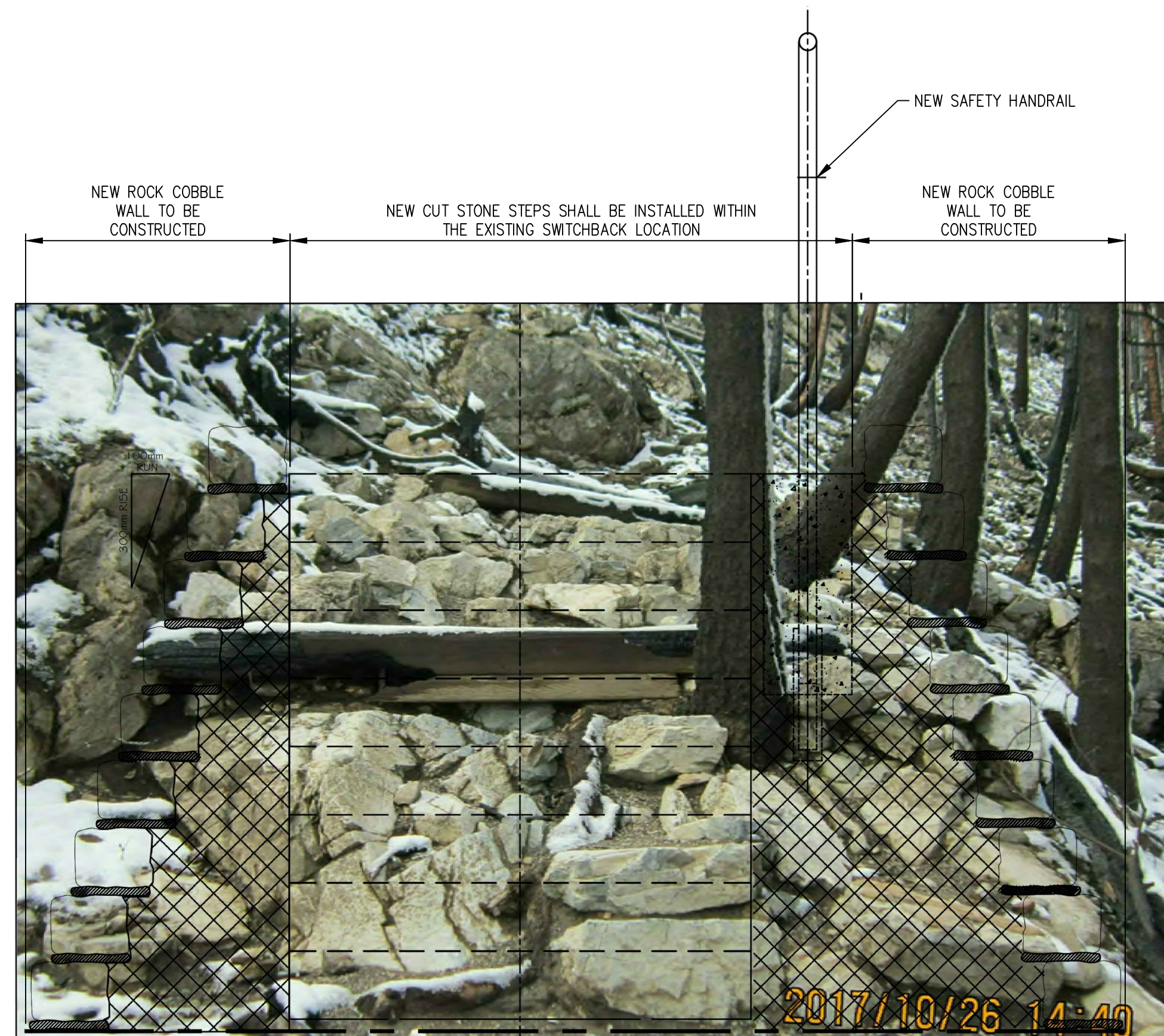
VIEW NTS EXISTING ROCK SWITCHBACK WITH IMPOSED CONSTRUCTION DETAIL
