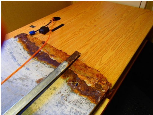
Figure 28: Corroded lower part of Joiner panel
