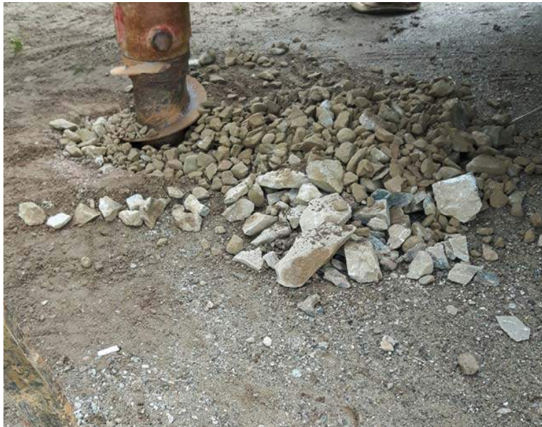
Visual of the cobble coming up during drilling.
