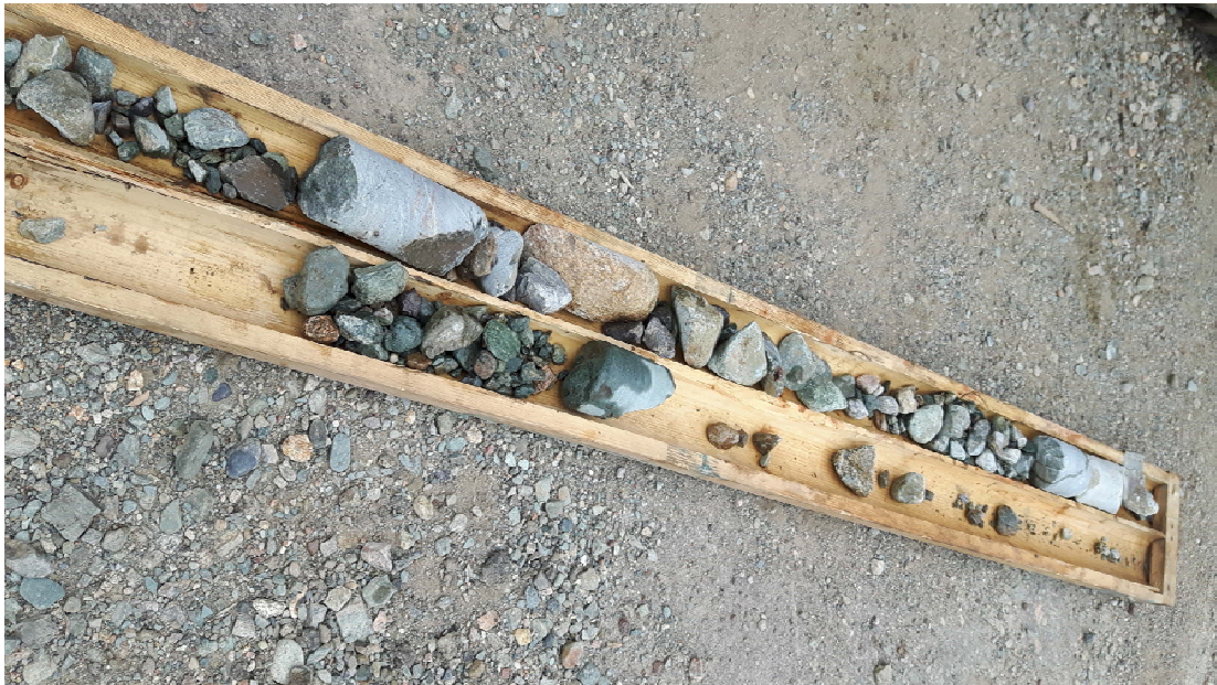
Cobbles and boulders cored from Borehole 3 (BH16-03).
