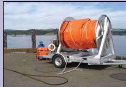
The hydraulic powered deployment reel with inshore containment boom available for requisition.
