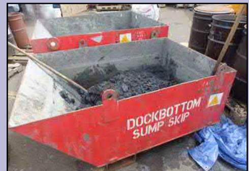
ADEQUATE waste grit storage.
