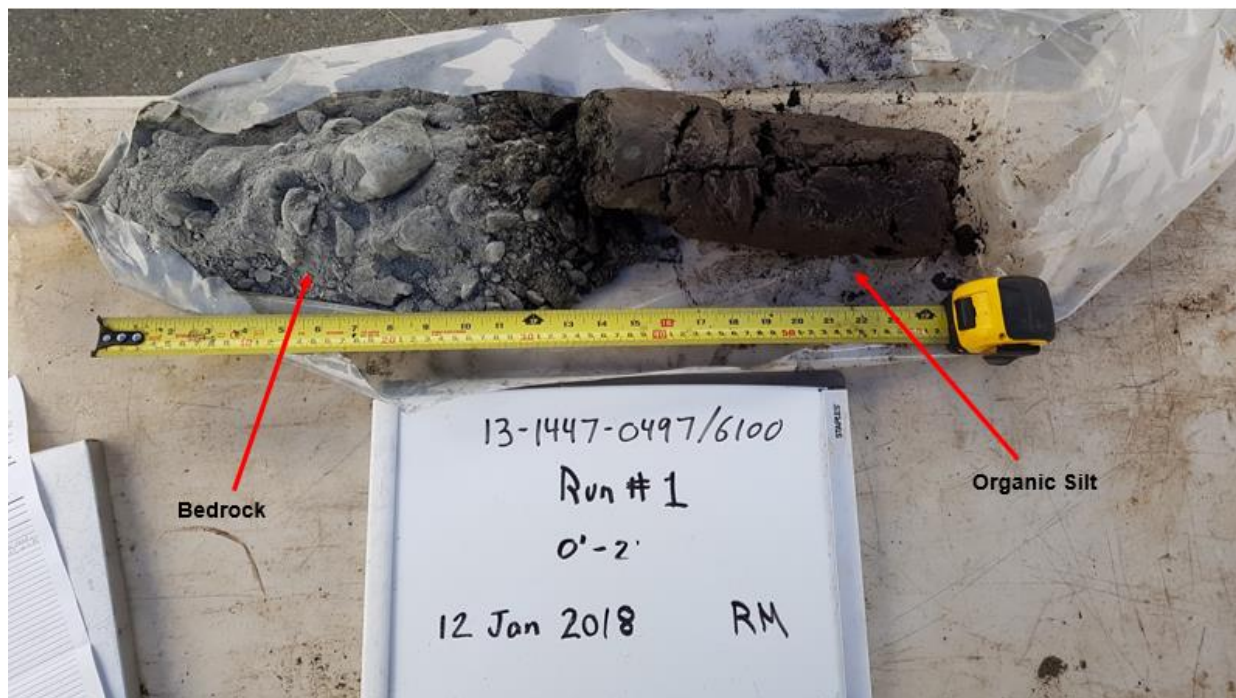
Photo 4: Example of sonic core sample from 0.0 m to 0.6 m at SDH18-02. Bottom end of sample is shown on the left side.
