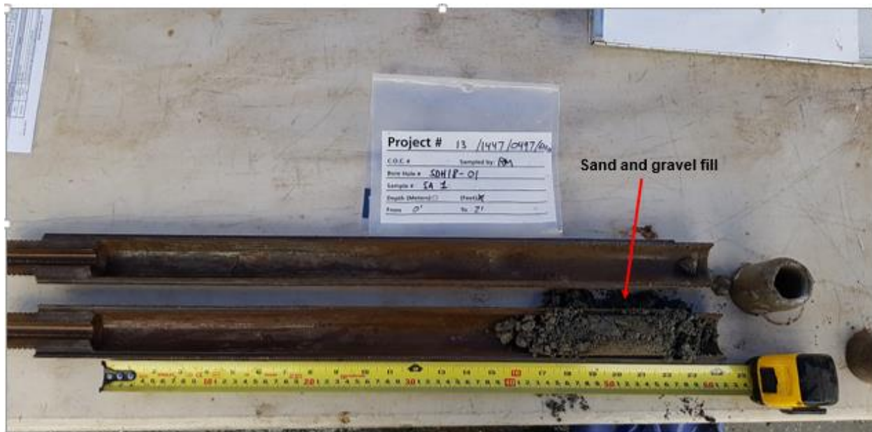
Photo 2: Example of a Standard Penetration Test split spoon sample at SDH18-01 from 0.0 m to 0.6 m.
