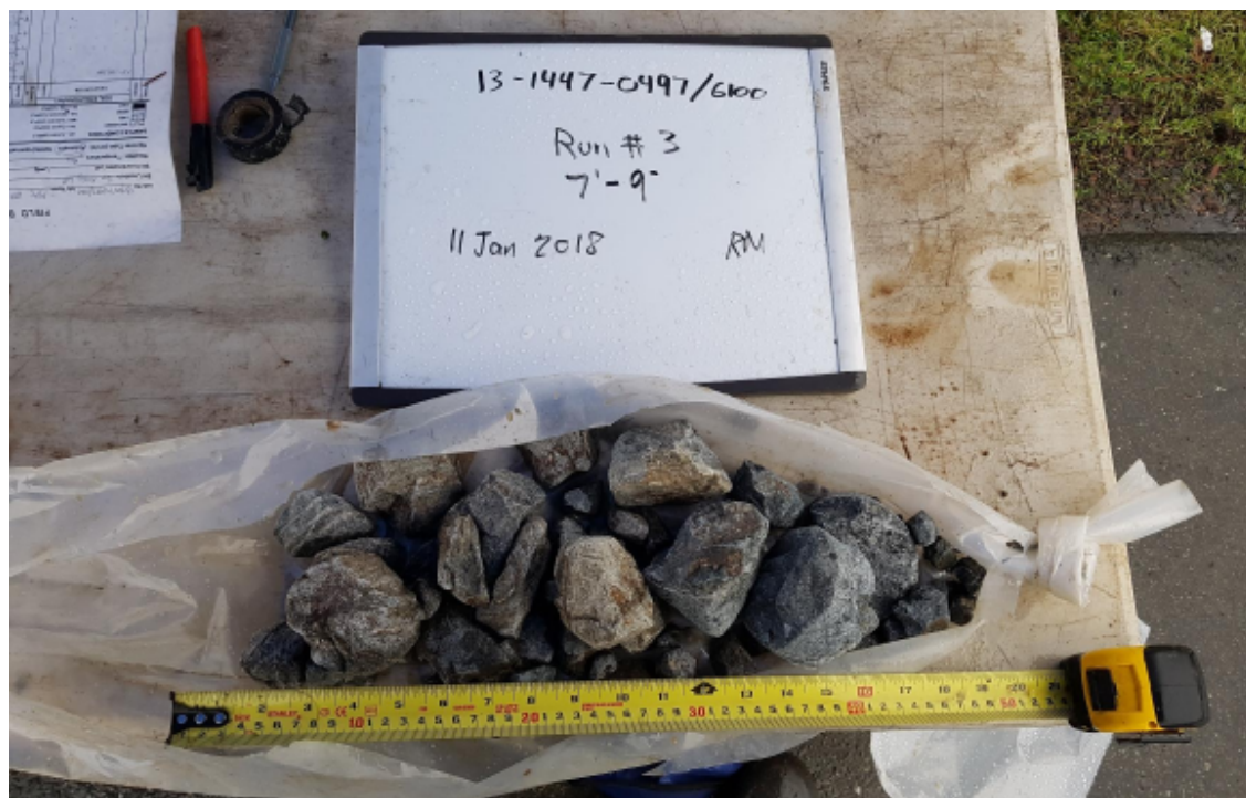
Photo 3: Example of bedrock from a sonic core sample from 2.1 m to 2.7 m at SDH18-01. Bottom end of sample is shown on the right side.
