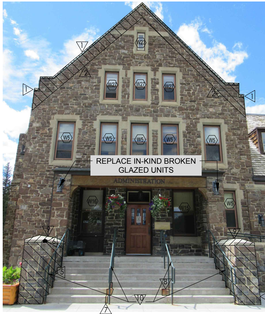
1 EAST ELEVATION-ENTRANCE A107
