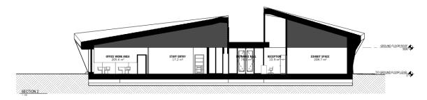
Figure 8. Amethyst Scheme Design Change - Reduce Net Air Volume
